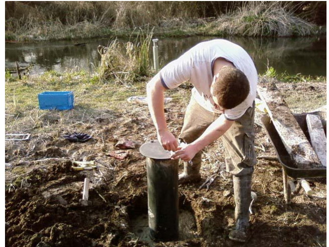
Figure 2.3 a) LO1 site: multi-level borehole, stilling well, and four river bed piezometers b) LO2 site: multi-level borehole and stilling well.
