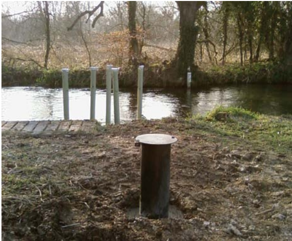
Figure 2.3 a) LO1 site: multi-level borehole, stilling well, and four river bed piezometers b) LO2 site: multi-level borehole and stilling well.
