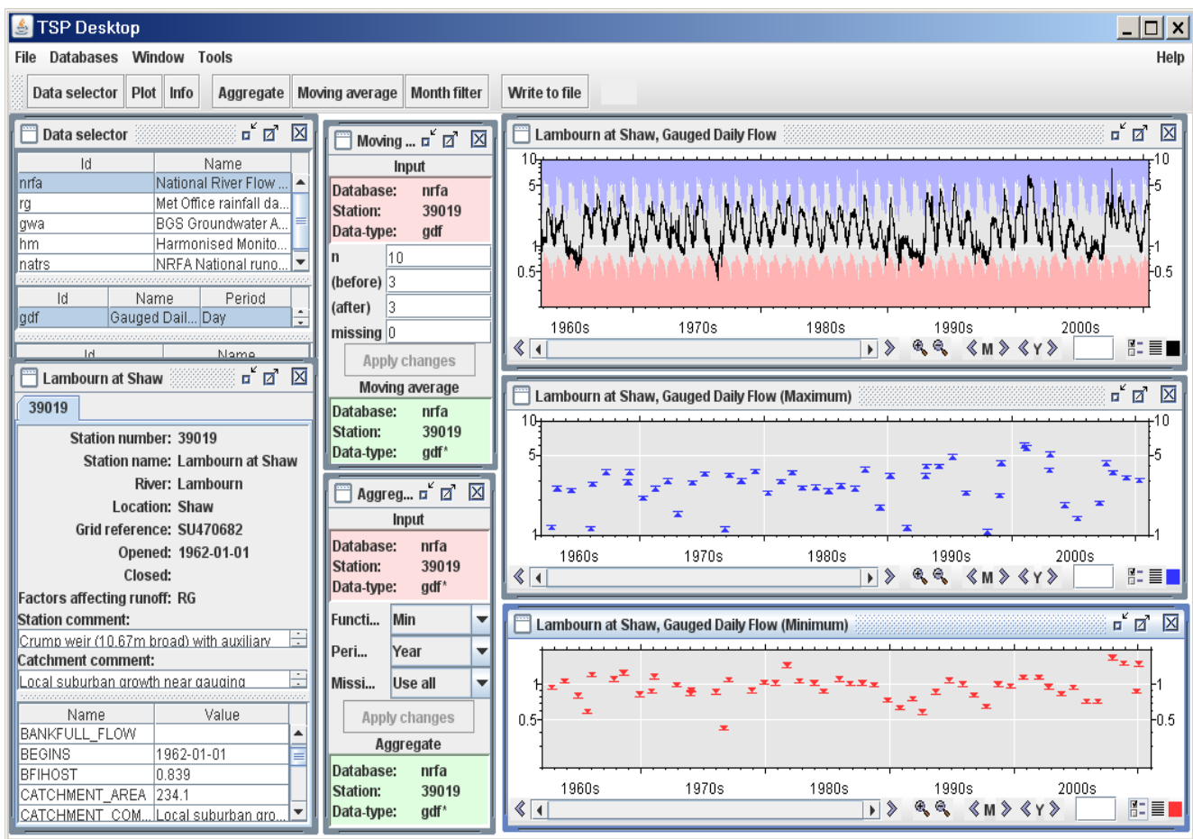
Figure 4 Shows the selection, manipulation and display of hydrological time series (and selected metadata) for a Benchmark Gauging Station. The plots show daily mean flows (with daily extremes indicated by the shaded envelopes) plus annual 10-day maximum and minimum gauged flows.
