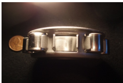
Figure 5 Small Inner Race Fault
