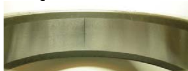
Figure 2 Small Outer Race Fault
