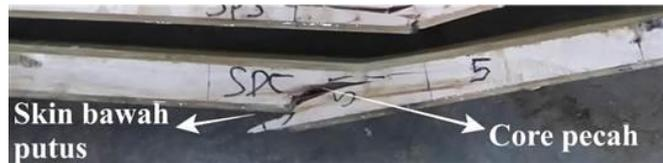
**Gambar 11. Pola Kegagalan Pada Balok Sandwich Panel SPS 5**
