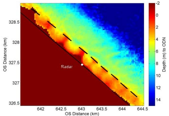
**Figure 3. A radar derived bathymetric map corrected to Ordinance Datum Newlyn (ODN) using a mean tidal level. The embayments are clearly defined and a set of subtidal dunes outside the breakwaters are evident.**
