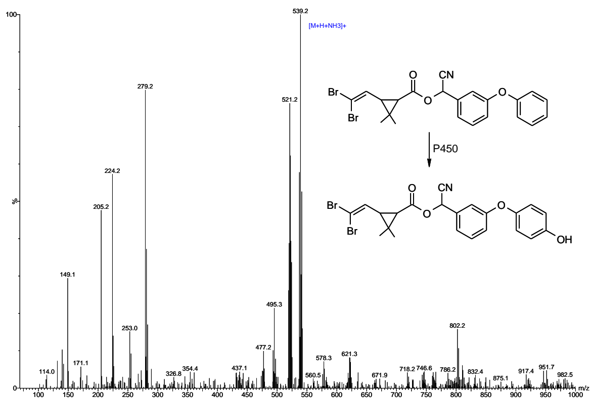
Fig. 27 Mass spectrum of 4-OH-deltamethrin. No other metabolites were detected in microsomal fractions of pollen beetle incubated with deltamethrin.
