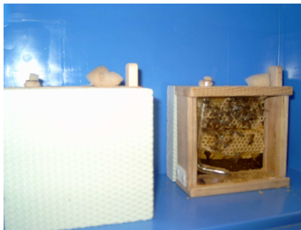
Figure 2.3 The cage bioassay: A wooden box with the dimensions 13 × 12 × 6 cm provided with a piece of wax comb and a feeding tube. A glass board enables the observation of queen-workers interactions.
