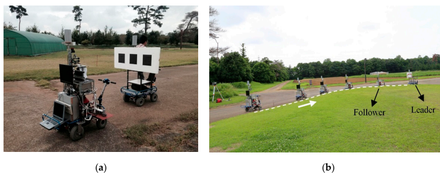
Figure 7. Field experiments of the leader-follower system. (a) Evaluation of the camera–marker system; (b) Tracking of a trajectory of the leader vehicle.
