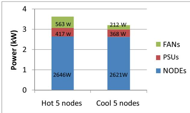
Fig. 17 Power consumption of node groups using LINPACK
