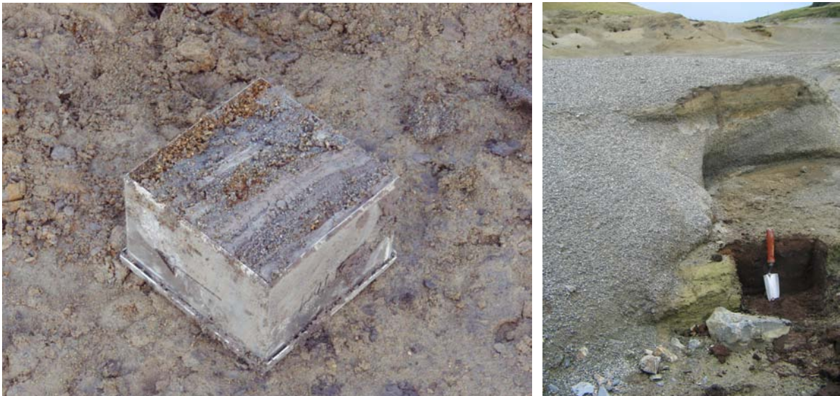
Figure 3: Kubiena tin sample showing variation in grading of the tailings. Figure 4: Peat exposed beneath the tailings.
