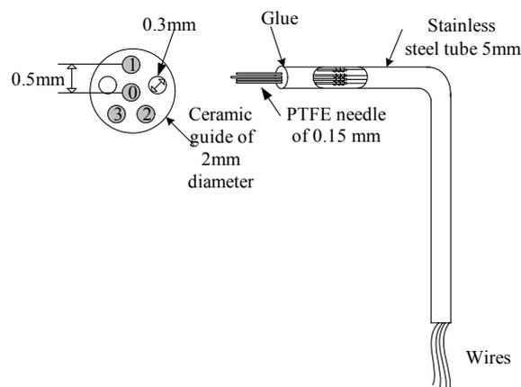
Fig. 1 Schematic of four-sensor probe
