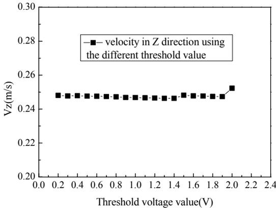
Fig. 7 The velocity of the bubble in the Z direction using the different threshold voltage values
