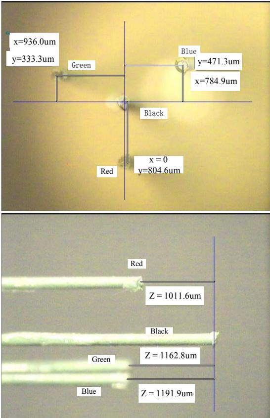
Fig.3 The 4-sensor probe viewed under a microscope
