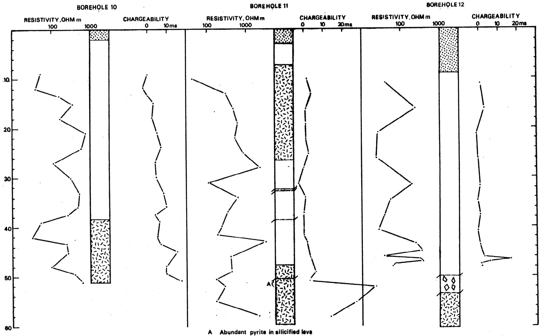
Fig. 11. Geophysical logs of boreholes 10, 11 and 12.
