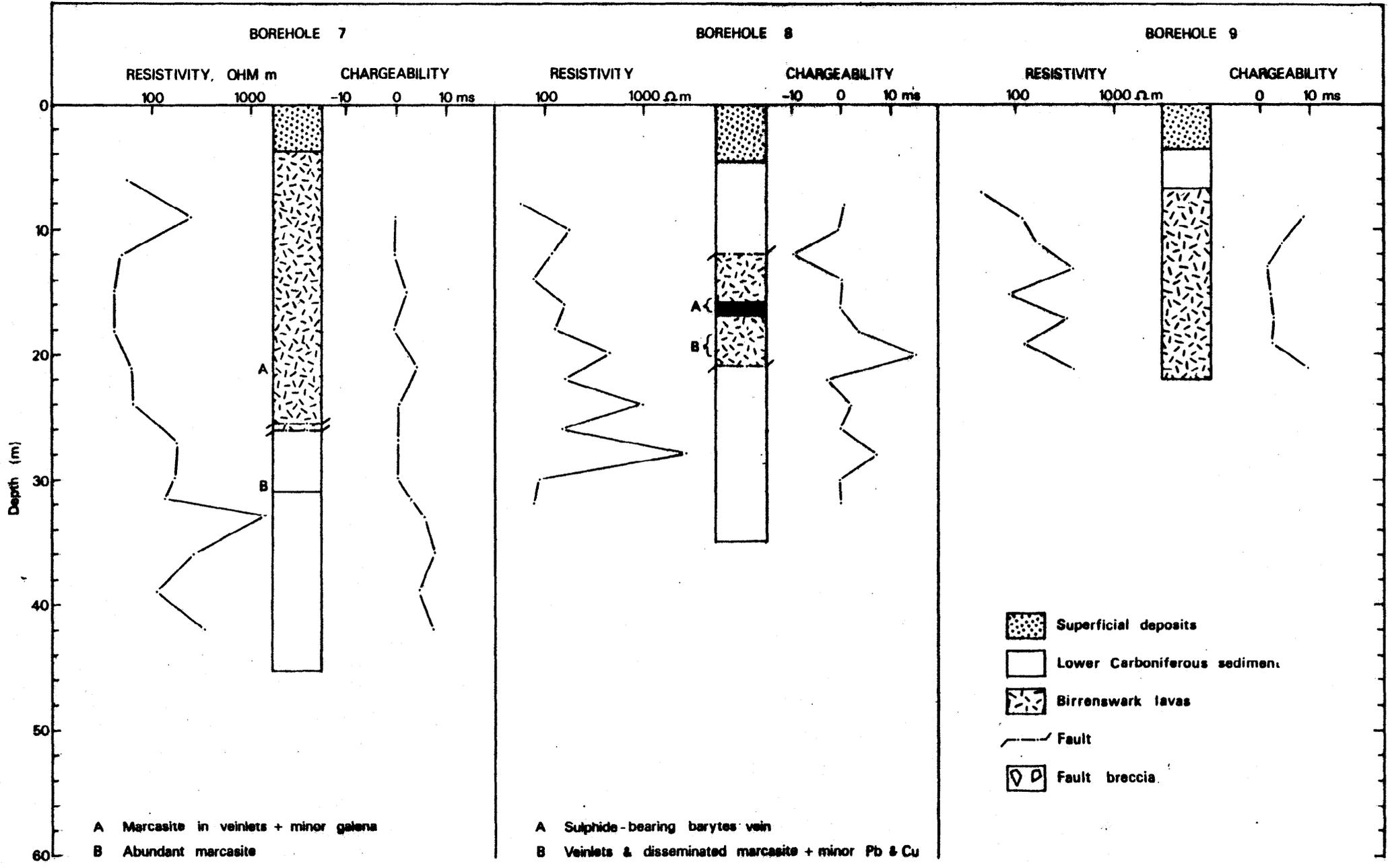
Fig. 10. Geophysical logs of boreholes 7, 8 and 9.
