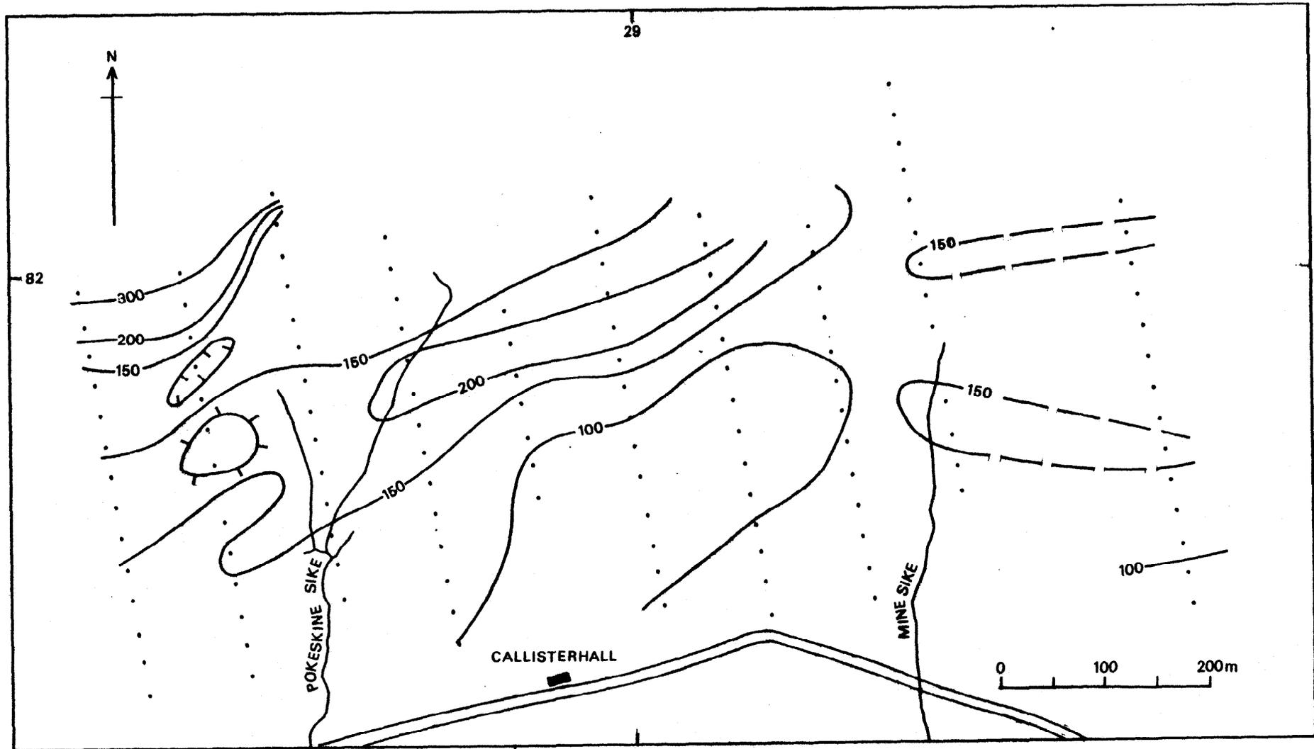
Fig. 7. Contour map of apparent resistivity in ohm metres, Callisterhall area, dipole-dipole array, with dipole centre-to-centre separation 60 metres.
