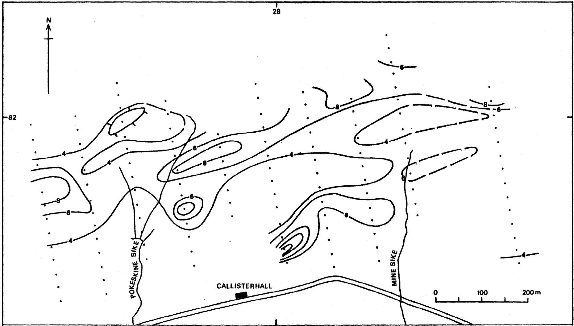
Fig. 8. Contour map of chargeability in milliseconds, Callisterhall area, dipole-dipole array, with dipole centre-to-centre separation 60 metres.
