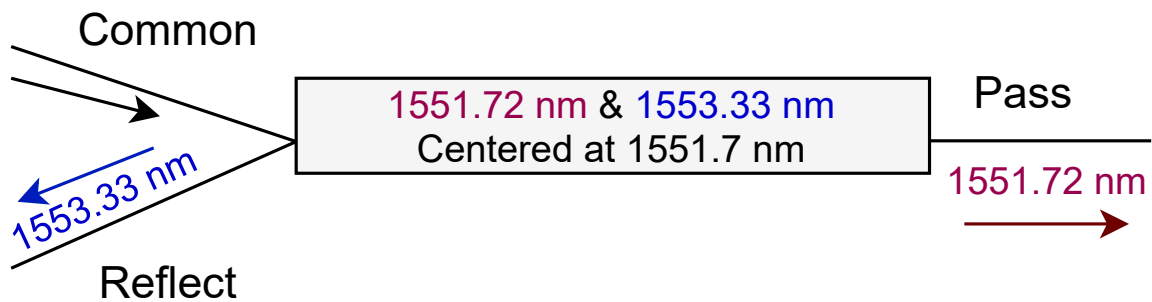
Figure 4.6: Illustration of a DWDM filter operation.
