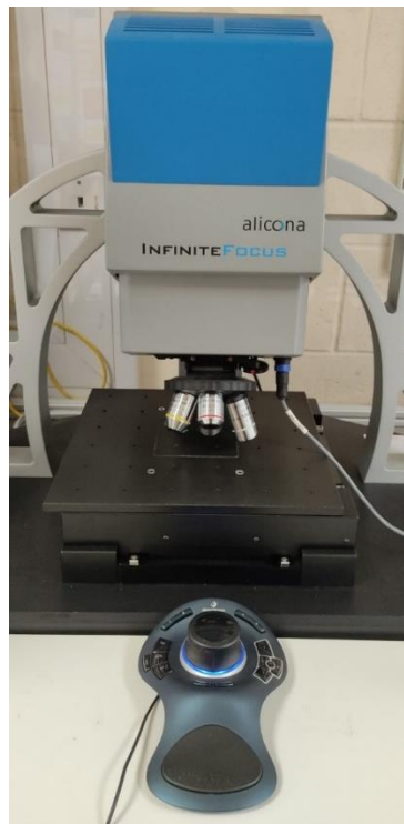
Figure 3.19 – Alicona InfiniteFocus G4 surface profilometer.
