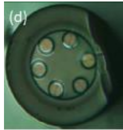
Figure 2.59 – Optical microscope image of free boundary anti-resonant hollow-core fibre [2.315].
