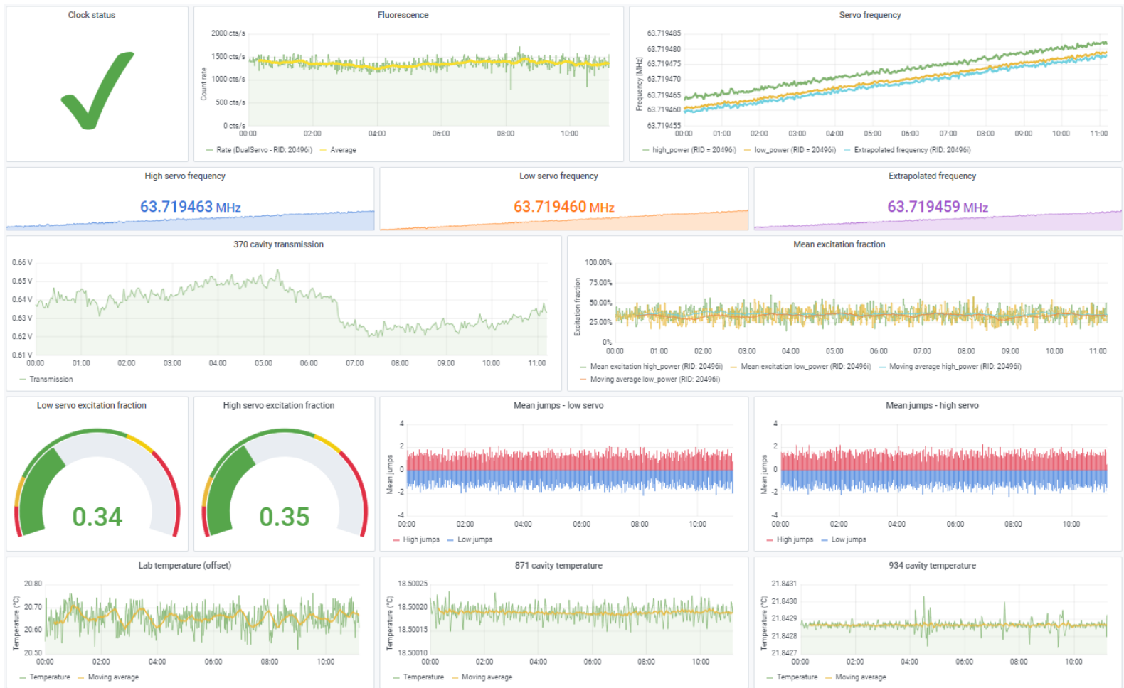
Figure 3.4: Grafana dashboard displaying data from a dual-servo lock experiment during a chosen time interval, showing ion fluorescence, clock servo frequencies, excitation fractions, high and low frequency jumps for high and low power servos, and laboratory and cavity temperature data.
