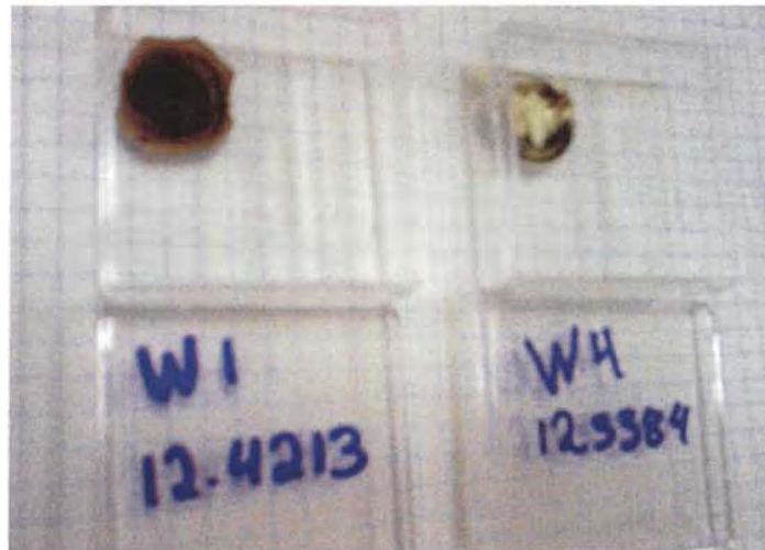
Figure 6.2 Two \text{WO}_3 samples: W1 (after heating) and W4 (before heating)
