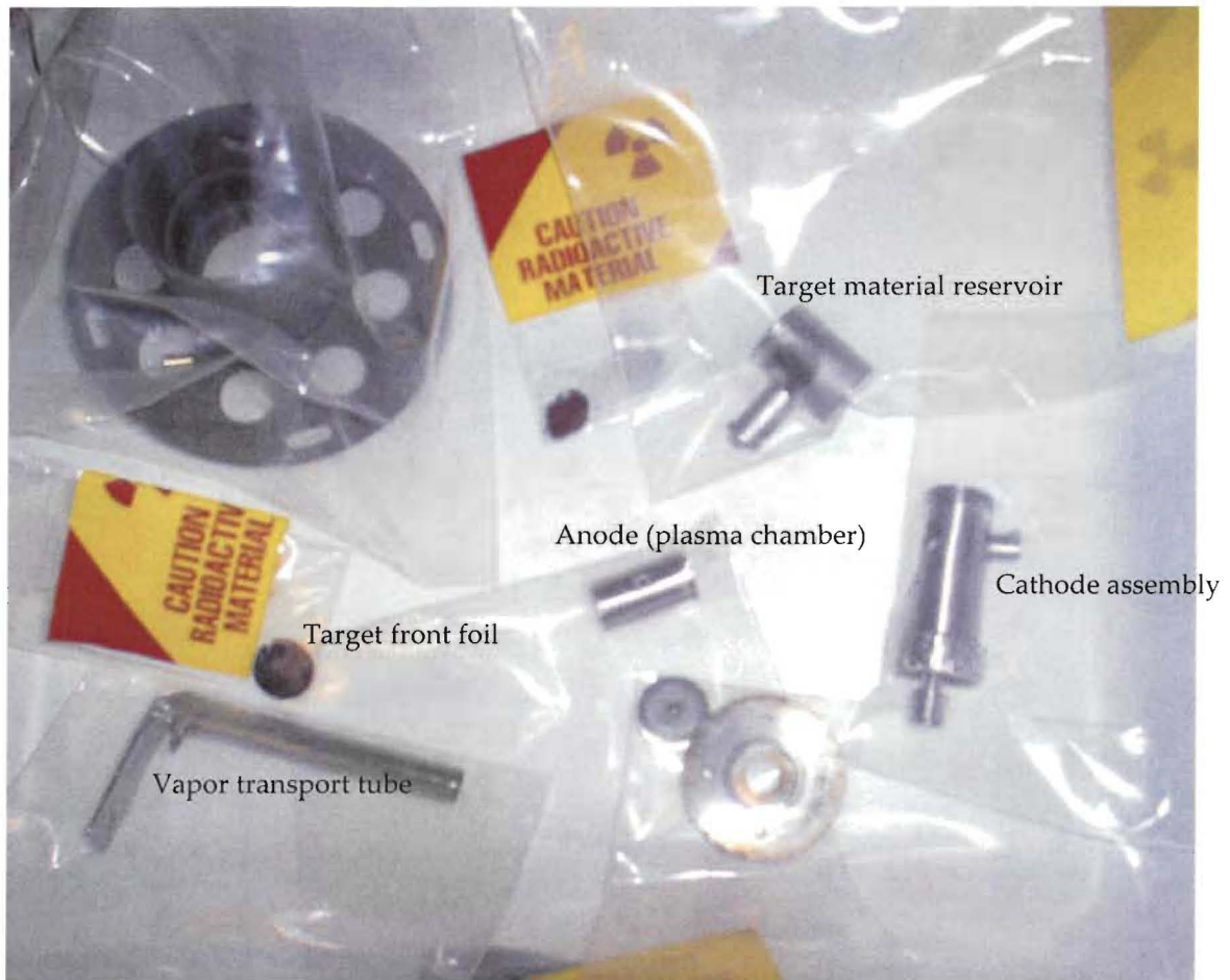
Figure 6.8 Photograph of the electron beam plasma ion source necropsy
