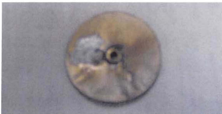
Figure 6.15 Faraday cup after one hour irradiation with 1.2 mA of H^+
