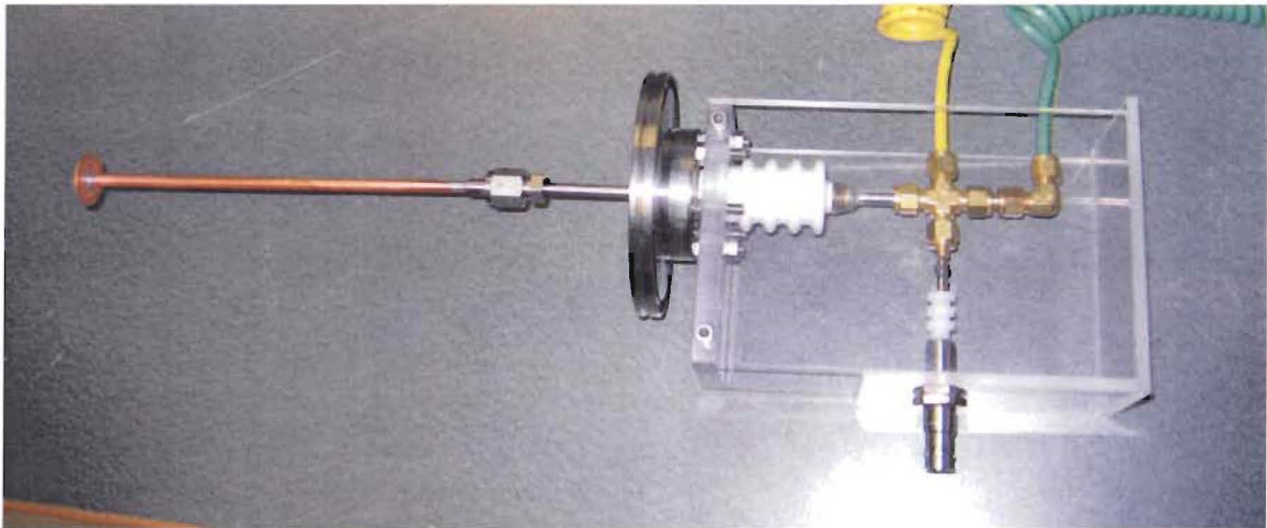
Figure 6.14 Water-cooled Faraday cup
