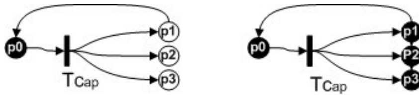
Figure 6.5: Petri Net pn_{ap} reachable firing sequence with input output domain connection.
