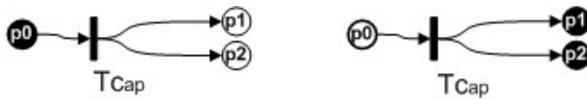
Figure 6.6: Petri Net pn_{ap} reachable firing sequence.
