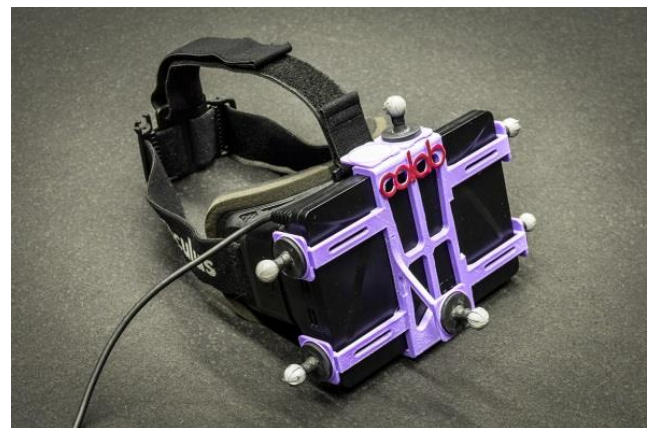
Figure 2. Headset with markers attached on a custom 3D printed mount.
