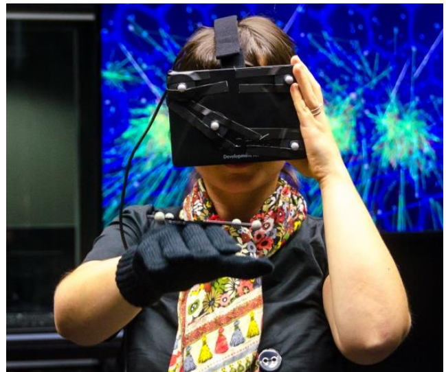
Figure 5. A user navigating through the virtual representation of the neural network and using an intuitive, hand position based 3D cursor for retrieving information about specific neurons.
