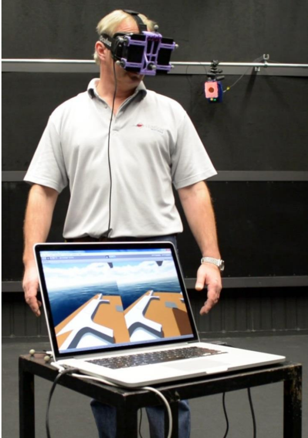
Figure 7. The yacht designer walking on the virtual representation of his CAD model.
