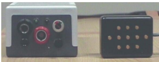
Figure 2. Three channel Laplacian electrode (right) and amplifier (left) used for data collection of sEMG signals from the vastus medialis muscle of the quadriceps. Supplied by Université de Technologie, Compiègne, France.
