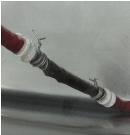
**Fig. 3.12** Platinum coated Nafion tube for first humidification experiments
