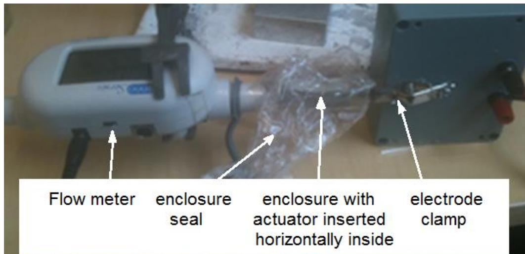
**Fig 3.10** Actuation Flow Rate and Chamber Shape Investigation
