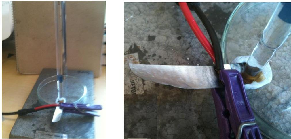
**Fig. 3.14** Pt-Nafion strip transverse hydration experiment third height version 305 mm
