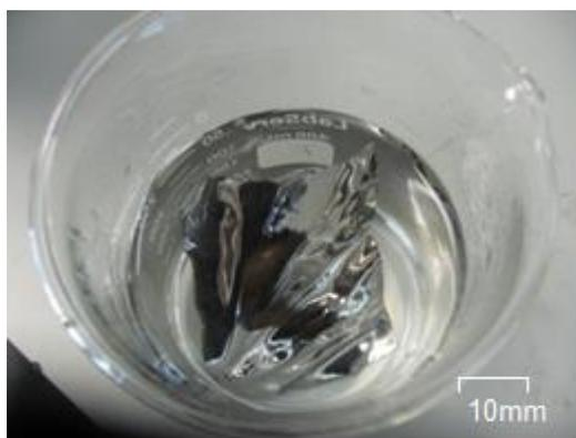
**Fig. 3.2** Smooth surface appearance of Nafion being platinum coated in solution
