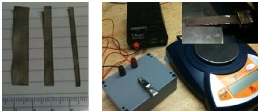
**Fig 4.6** Nafion beam samples and DC source, fixture and scale for force
