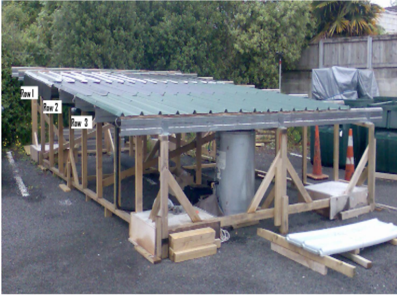
Fig. 5: Glazed BIT Test Rig
