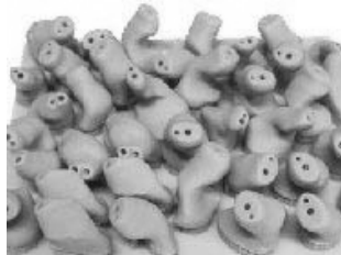
Figure 5. Individually customized hearing aid shells mass-produced by an EOS laser sintering system. Special CAD software has been developed by Materialize to make the process of converting the customers' ear canal laser scan data into the product easy and seamless. Reproduced with permission, The Hearing Review, USA.
