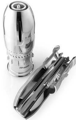
Figure 3. Fuel Injection Swirler (made out of Cobalt Chrome MP1) from Morris Technologies. This part would be impossible to cast but can be easily made through additive manufacturing. Reproduced with permission, Morris Technologies, USA.
