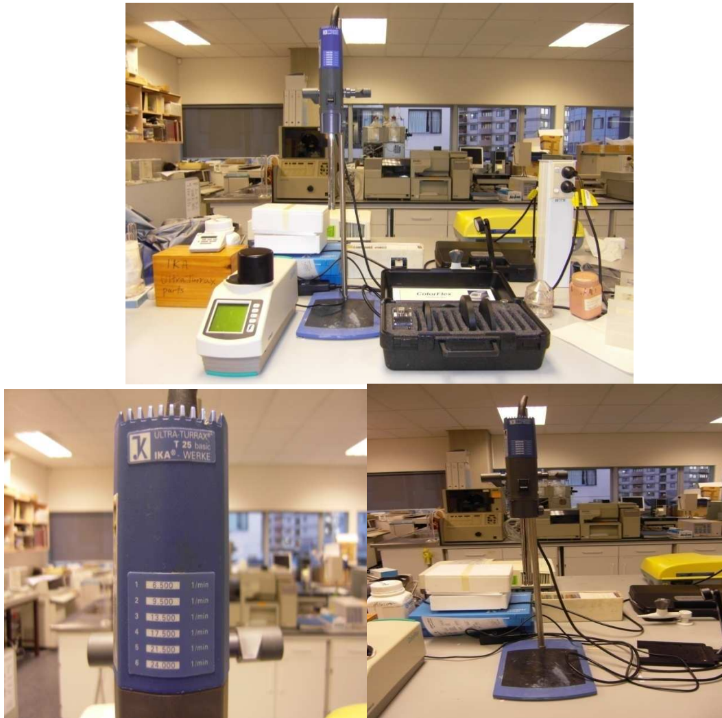
Figure 14. Homogenizer (Ika T25) basic Ultraturrax fitted with a dispersing element.
