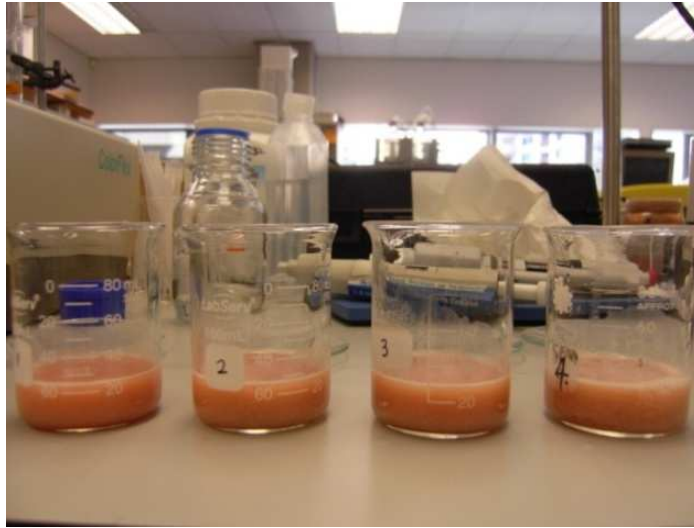
Figure 11. Colour of muscle slurries containing different concentrations of glucose, but no Fehlings' solution. The glucose concentrations were, from left to right, 6.67, 3.34, 1.22 and 0 mM. (From Lei, 2009).
