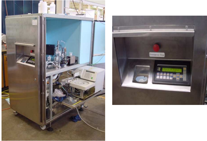
Figure 7. An exposed view of a semi-automatic machine to measure liberated glucose in a small pre-rigor muscle sample. The sample is placed in the hole on the fascia of the machine. (Picture courtesy of Dr. O.A. Young.)
