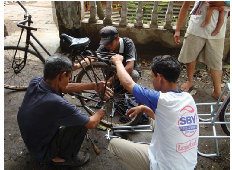
Figs 264 & 265. Putting the trailer attachment onto the bicycle
