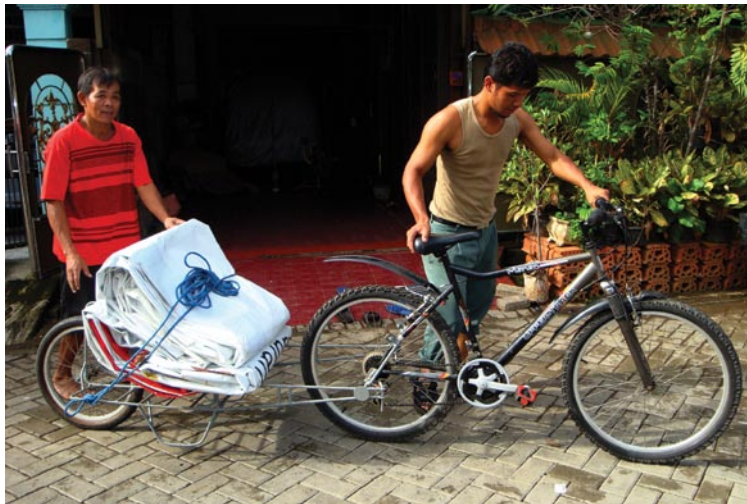
Fig 243. Trailer testing with a 100kg load
