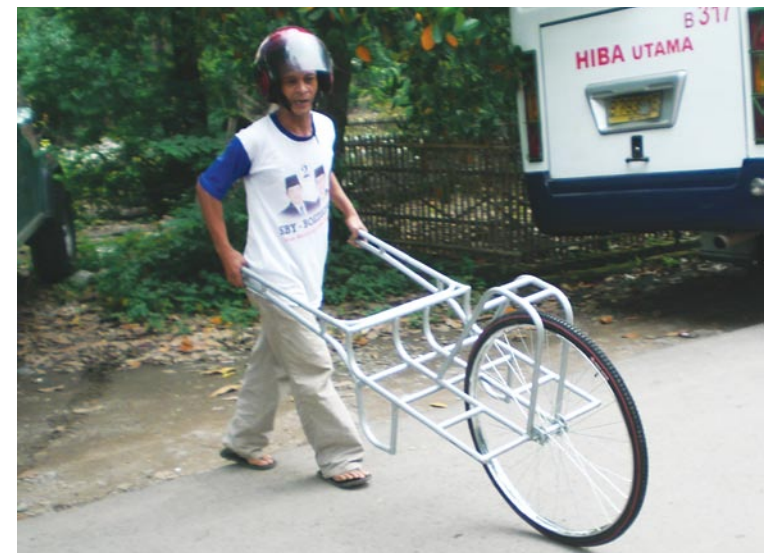
Figs 280-282. Locals testing the trailer as a wheel barrow
