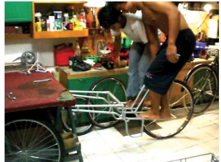
Fig 252. Testing the wheel and tyre
