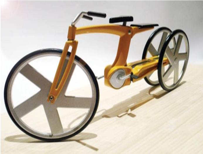
Fig 206. Front view of rapid prototype semi-working scale model with rear with rear arms close together
