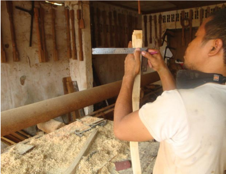
Fig 84. Bamboo strips measured to the required size
