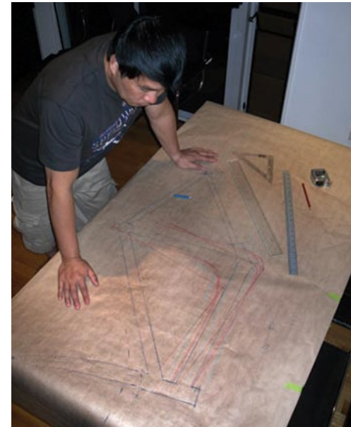
Fig 127. Producing the full-scale Greencycle frame pattern
