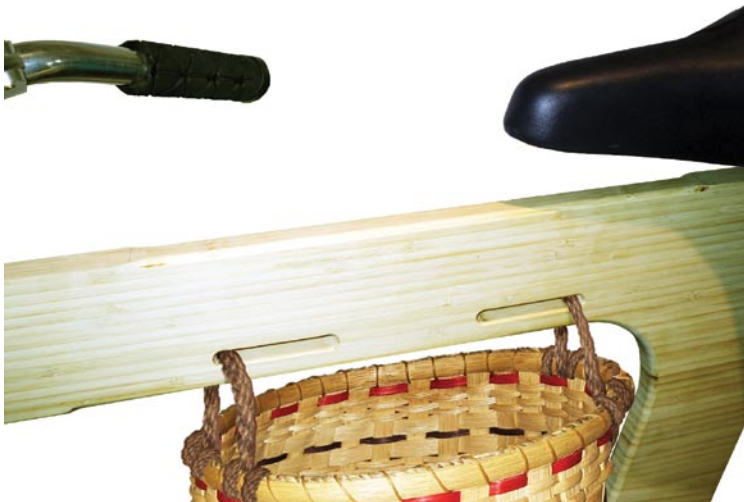
Fig 119. How slots can be used for basket attachment
