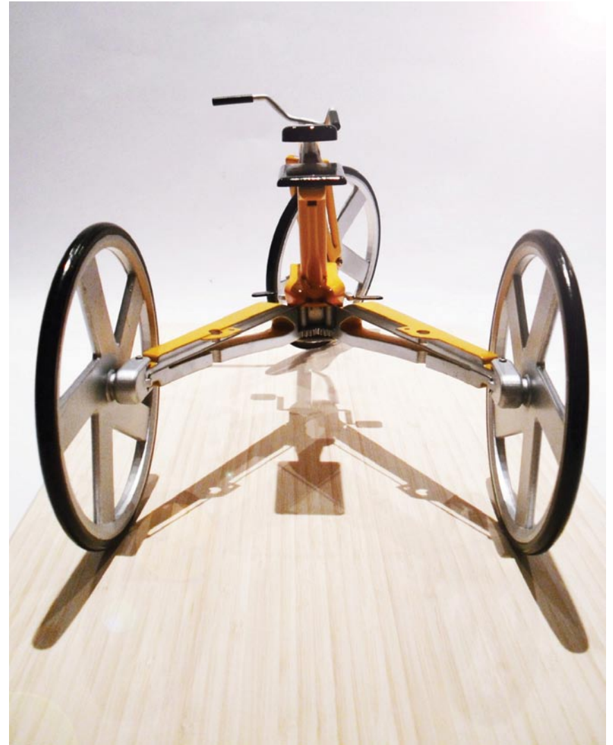
Fig 205. Rear view of rapid prototype semi-working scale model with rear arms splayed apart
