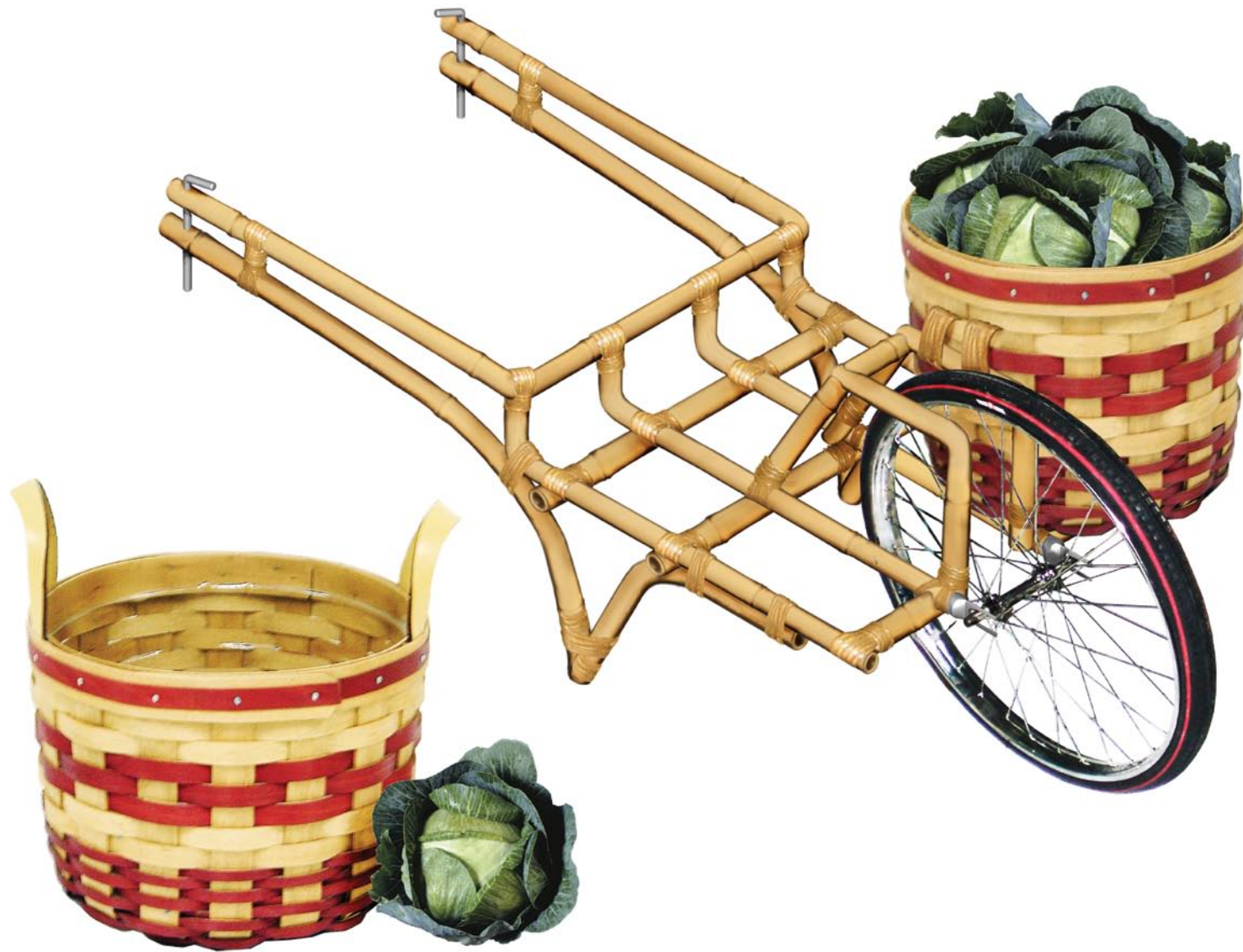
Fig 195. Envisaged bamboo trailer with woven bamboo baskets
