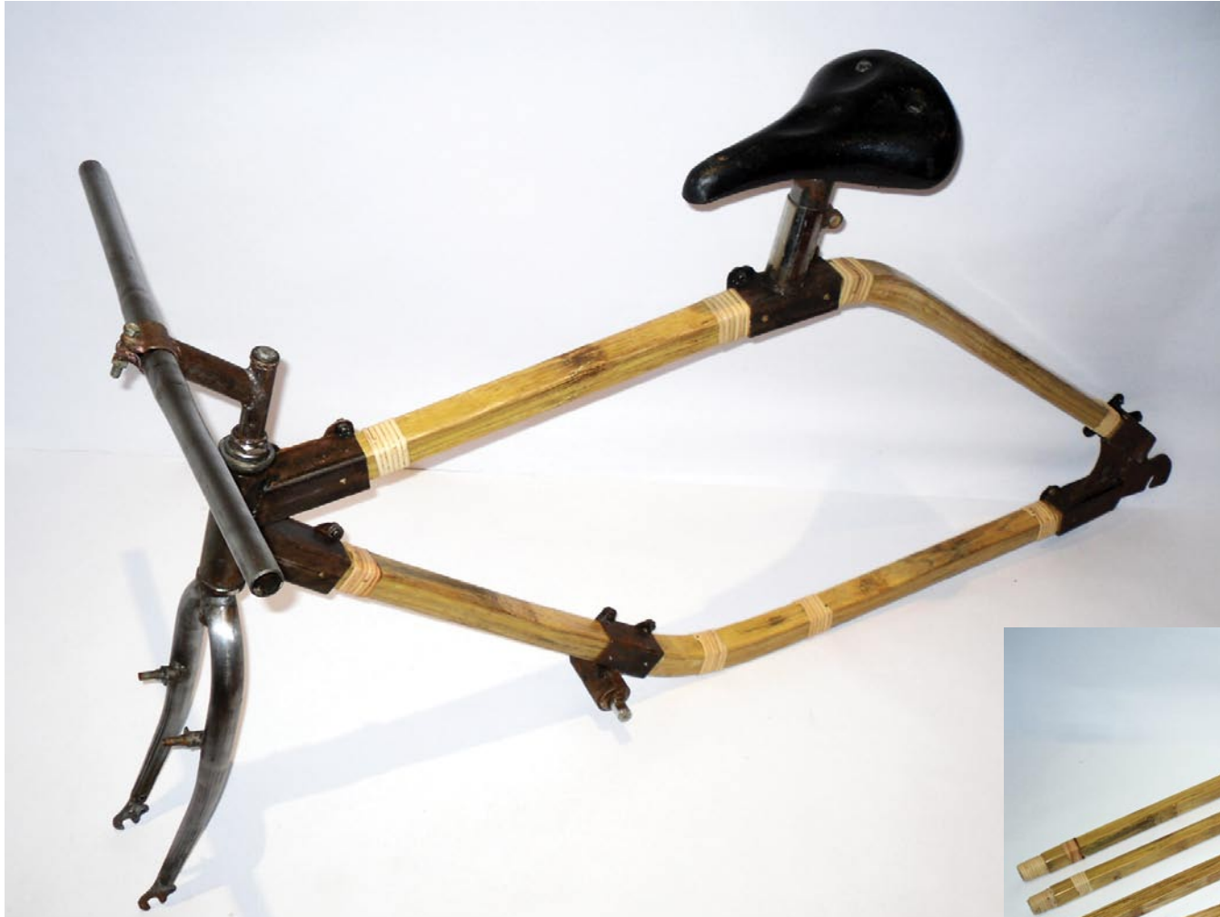
Fig 107. Complete bamboo laminated frame no.2
