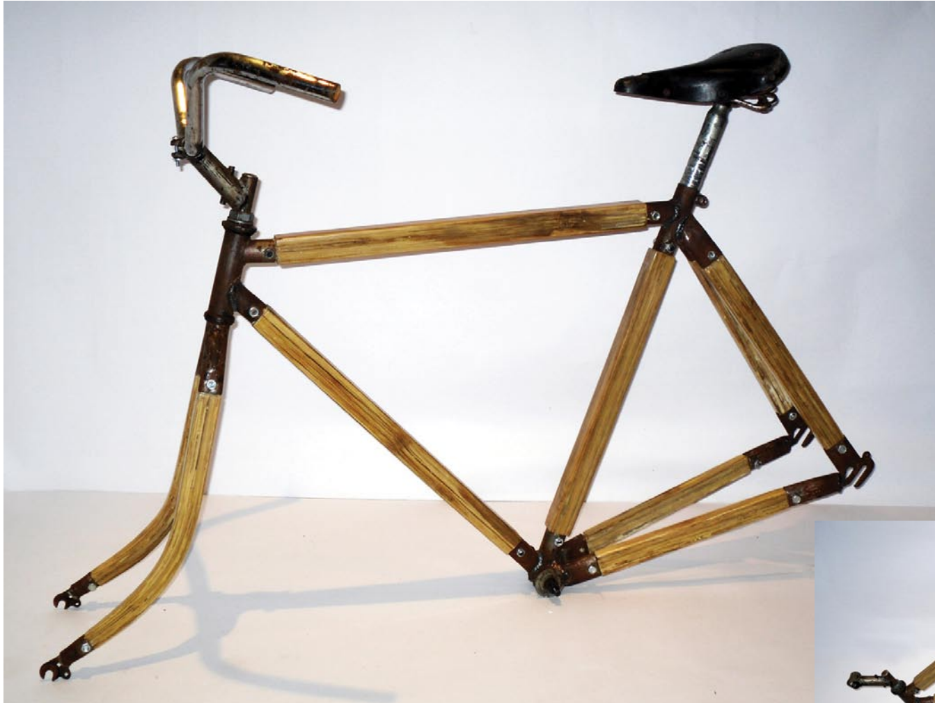
Fig 97. Complete bamboo laminated frame no.1
