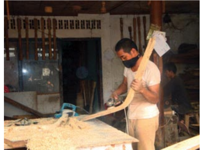
Fig 85. Bamboo strips cut to the required size
