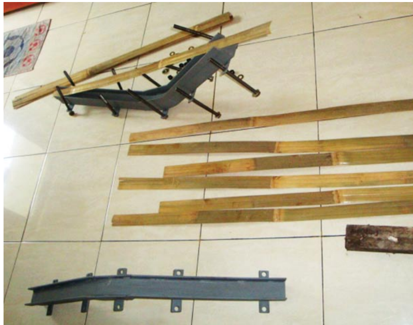
Fig 81. Bamboo strips on two-piece steel mould
