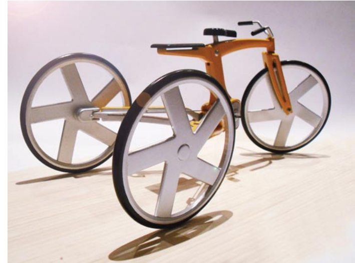
Fig 207. Rear view of rapid prototype semi-working scale model with rear arms splayed apart
