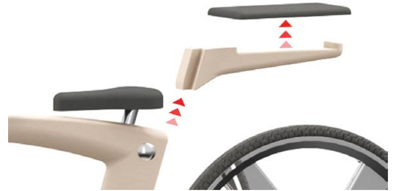
Fig 202. CAD rendition of the multi-function rear seat structure
