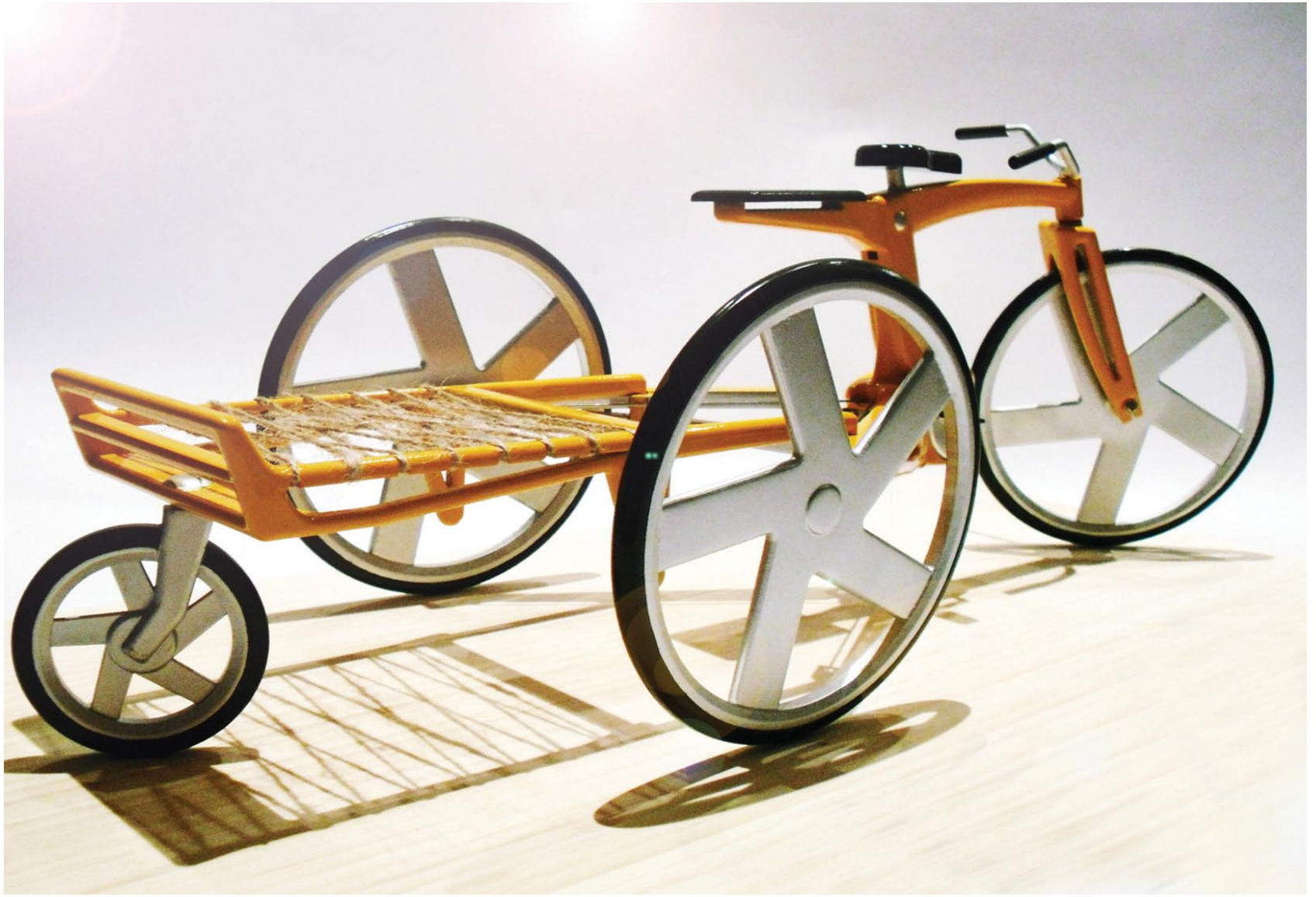
Fig 210. Rear View of rapid prototype semi-working scale model of the ideal bicycle with the multi-function trailer
