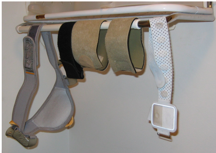
Illustration 4: Sensor & iPaq mounts after washing - iPaq belt on left (plastic holder for iPaq is at bottom), sensor mounts are two brownish straps, strap on right is battery holder for an early version of the SF sensor.
