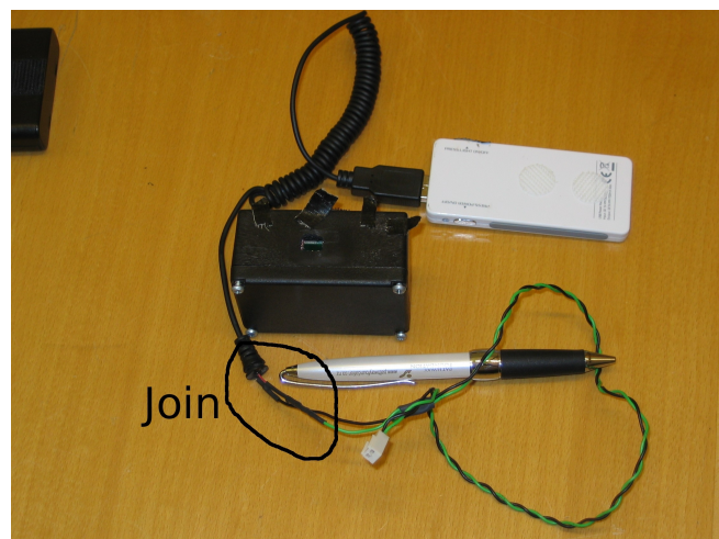
Illustration 11: SF sensor, USB battery & cable. The joint where the cable broke is circled
