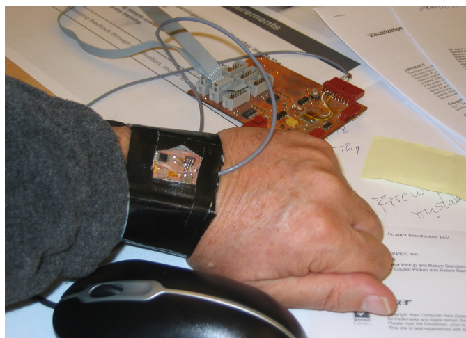
Illustration 1: An early prototype based on a modified SmartBadge platform
