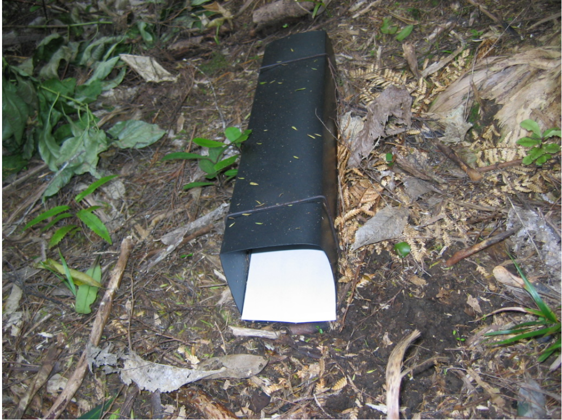
Plate 2-4 Black trakka™ tracking tunnel containing card for rodent monitoring.
