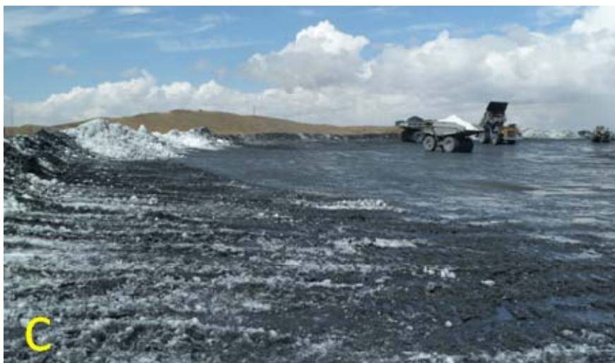
Figure 37 (A): Kumtor Gold Mine open pit, 4000 m a.s.l.; (B): removing of Davydov glacier in order to get to the gold bearing rocks ; (C): Redepositing of glacier ice. Source: July 2011, M. Duishonakunov.
