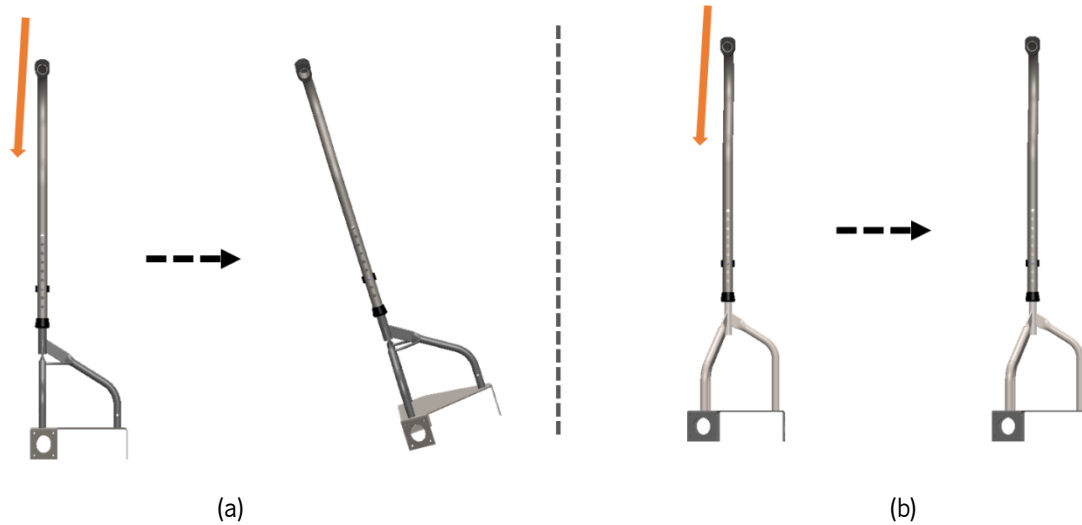
Figure 3.11: Example of forces applied vertically in: (a) the primordial design of the ARCcane, resulting in falling over, due to a decompensation between center of mass of the structure and the forces applied by the user on the ARCcane handle; (b) the new structural design of the ARCcane, where the handle is placed right above the ARCcane center of mass, having smaller impact in the stability of the structure.
