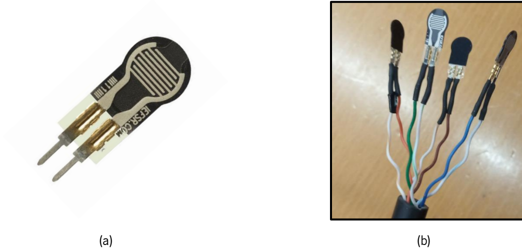
Figure 4.9: (a) One and (b) the combination of four Interlink FSR® Model 400 Short Tail force sensors used as an axial force system.
