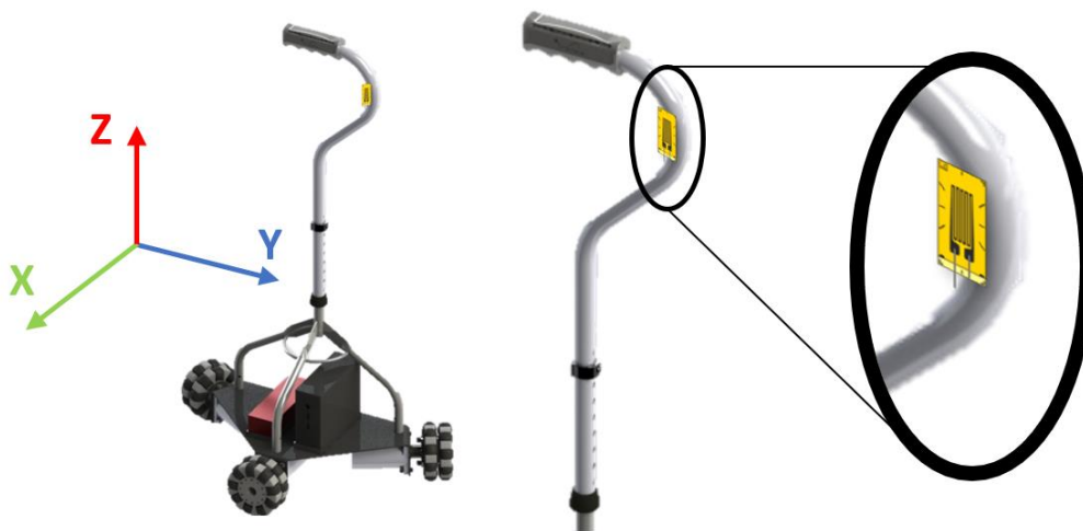
Figure 6.6: Proposed strain gauge sensor configuration to obtain a gait phase detection sensor, which allows detecting the forces applied to the cane in the z-axis direction.
