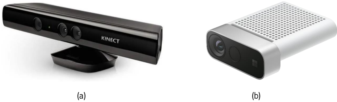
Figure 7.6: (a) Microsoft Kinect (discontinued manufacturing). Image from [171]; and Microsoft Azure Kinect. Image from [161].
