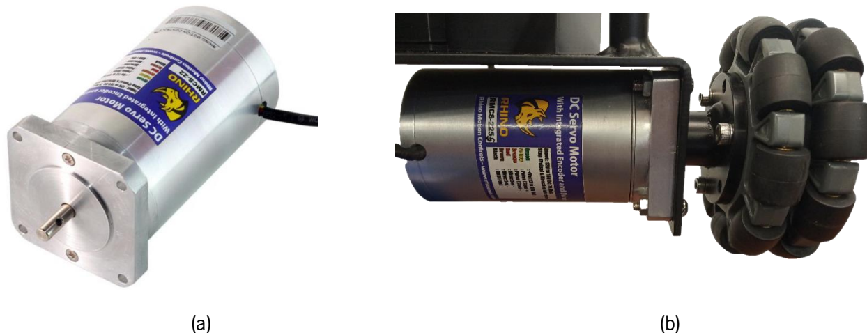
Figure 4.23: (a) DC Servo motor NEMA23 (RMCS-2255) by Rhino Motion Control Solutions. Image from [130]. (b) Insertion of the motor into the holonomic base of the cane.
