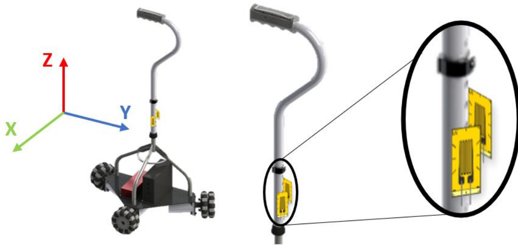
Figure 6.5: Proposed strain gauge sensors configuration to obtain an axial force system, which allows detection of movement intent in both x-axis and y-axis directions.
