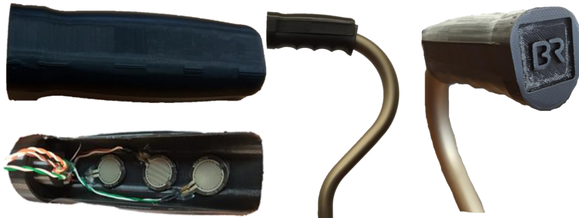
Figure 6.16: Visual representation of the 3D structure with the insertion of the three haptic force sensors with its implementation in the ARCanE handle.
