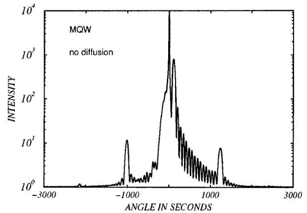
FIG. 3. Simulated Cu  $K_{\alpha_1}$  004 DCXRD rocking curve for  $15 \times 80$  Å CdTe wells separated by 80 Å Cd<sub>0.925</sub>Mn<sub>0.075</sub>Te barriers with no diffusion.
