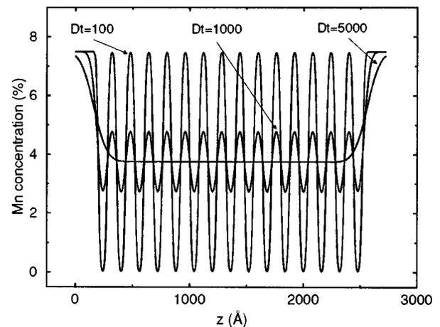
FIG. 4. Diffusion profiles for the sample of Fig. 3 with varying values of  $Dt$  (in Å<sup>2</sup>).
