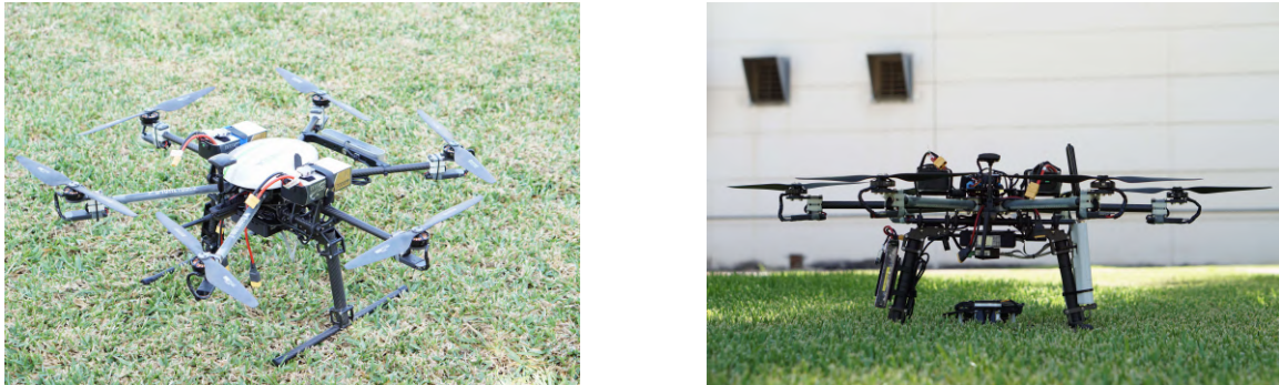
Figure 5.7: Aerial platform developed for the Challenge. Left, airframe without the mission electronics and the pickup mechanism. Right, fully equipped hexacopter.
