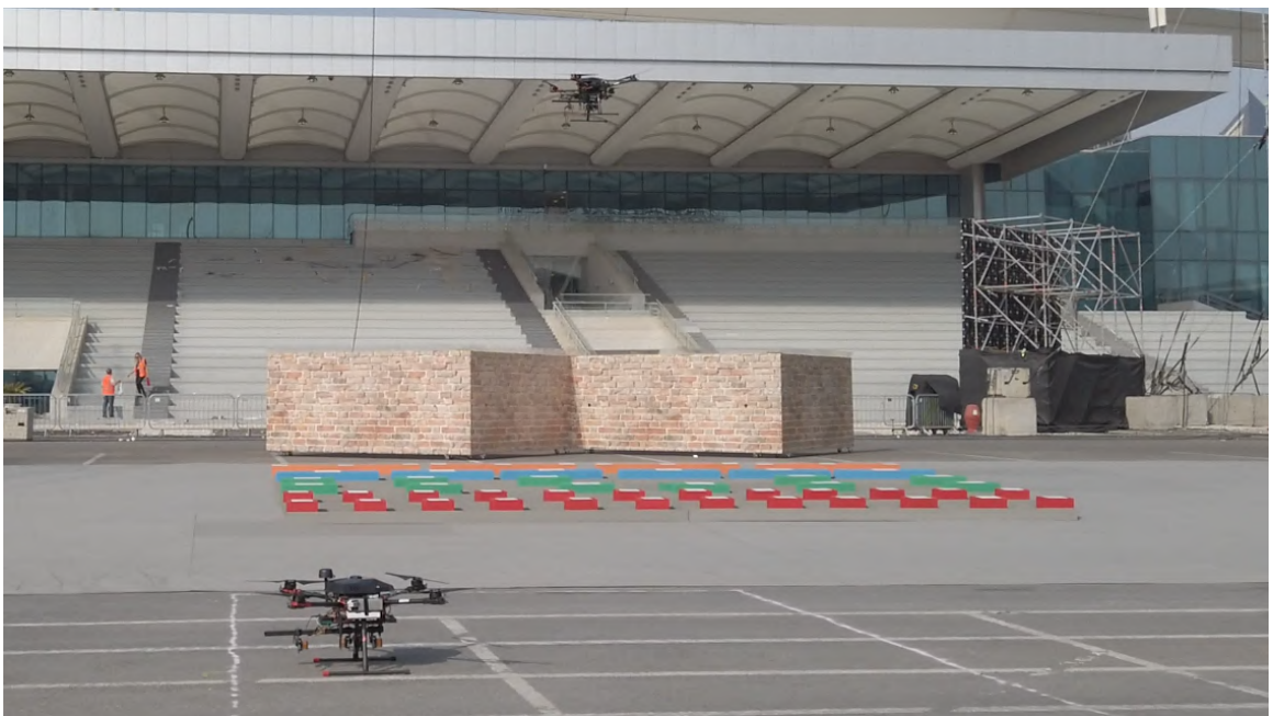
Figure 6.1: View of the arena for the MBZIRC Challenge 2. The structure to build Wall 2 has four segments, and the piles of bricks for the UAVs can be seen in front of the wall.
