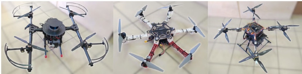
Figure 2.1: Examples of a foldable quadcopter (left), a hexacopter with tilted rotors (center), and a coaxial octocopter (right).
