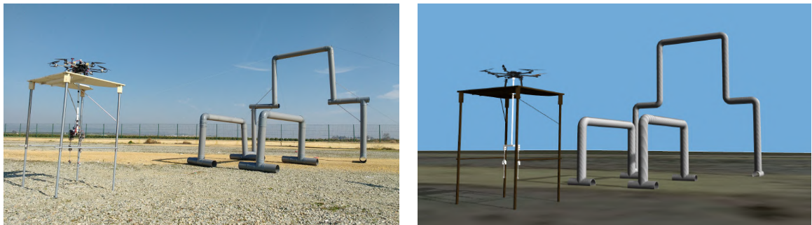
Figure 1.3: Experiments for aerial manipulation in a mockup scenario emulating pipes in a plant. A real and a simulated environment are depicted.
