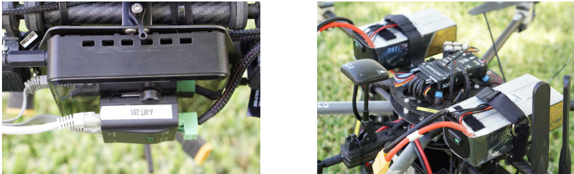
Figure 5.9: Detailed view of the core of the aerial platform. Left, Intel NUC computer with plastic case. Right, Pixhawk autopilot on top of the damped base.
