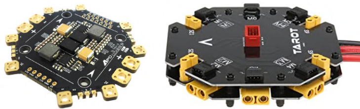
Figure 2.6: Examples of two different Power Distribution Boards.
