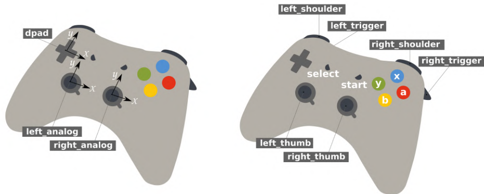
Figure 3.6: Layout for a standard joystick. Left, the 6 axes used; right, the 12 buttons used.
