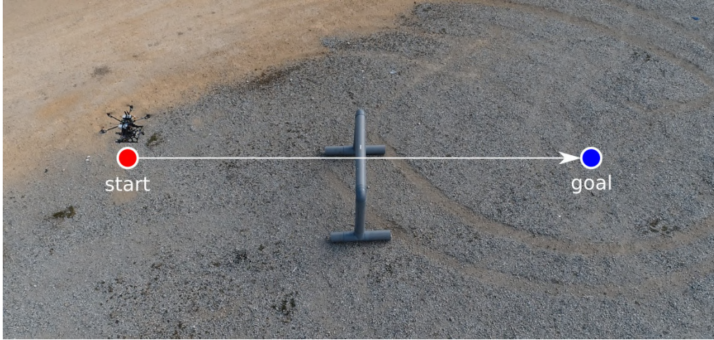
Figure 4.22: Scenario for field experiments. The start position is depicted in red and the goal position in blue. A non-mapped U-shaped pipe is placed between both locations.
