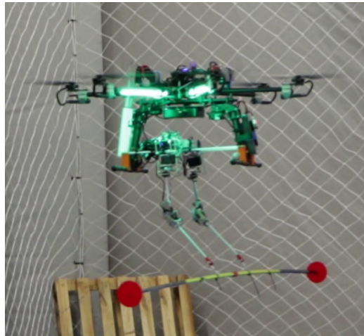
Figure 4.2: ARS platform designed for the AEROARMS project.
