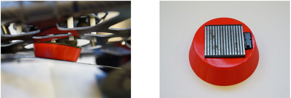
Figure 5.10: Prototype of the pickup mechanism. Left, detail of the damped platform. The EPM is grabbing a metallic disk and it has a certain degree of flexibility. Right, the holder with a single EPM and a contact sensor.
