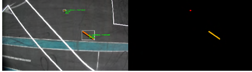
Figure 5.4: Output of the vision-based object detector. Left, original image from the arena with a red and an orange object. Bounding boxes and a text displaying extra information overlay the image. Right, processed image after the color segmentation. The two objects appear segmented and the background as black.
