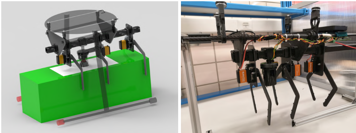
Figure 6.19: Left, rendered view of the grasping mechanism with a green brick. Right, real implementation.
