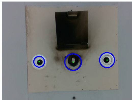
Figure 6.10: Output of the Hole Detector. The facade fire is not active but its central fire ring is detected with the RGB-D camera. The additional holes to simulate wind gusts are the same size and hence also detected.
