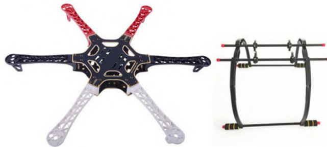
Figure 2.5: Examples of a hexacopter frame (left) and a landing gear (right).
