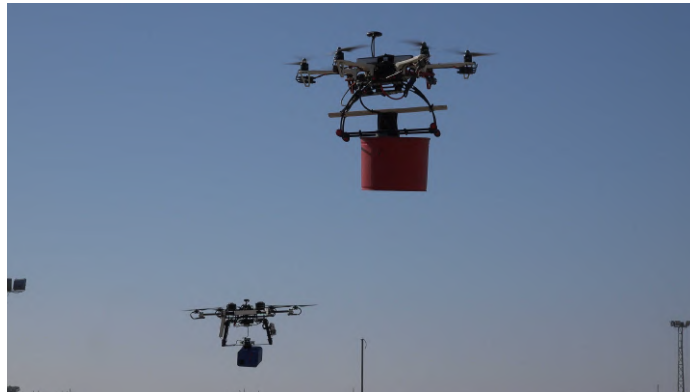
Figure 5.11: Preliminary tests in Seville (Spain). A DJI F550 aerial platform with our pickup mechanism transporting a red object (top) and our final custom-made hexacopter transporting a blue object (bottom).
