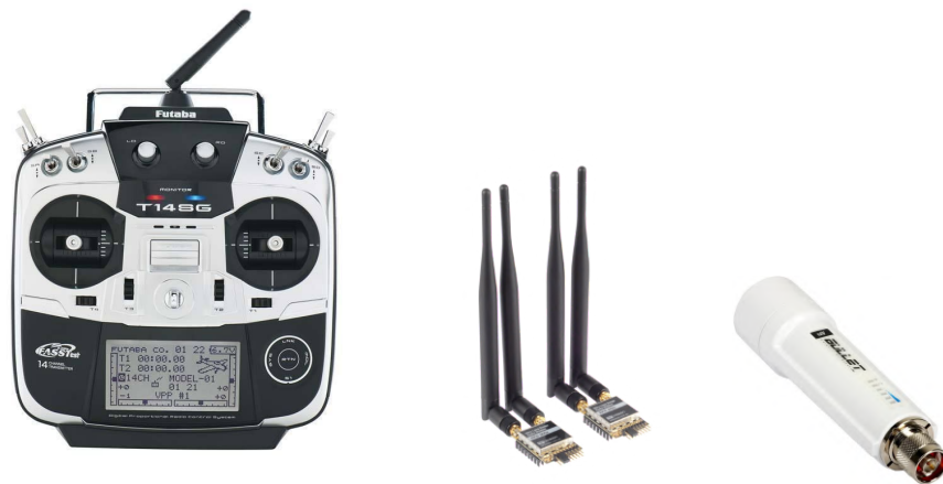
Figure 2.11: Communication device examples, from left to right: Futaba RC transmitter, a pair of 900 MHz radio modems, and the Ubiquiti Bullet M.
