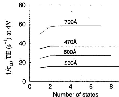
FIG. 11. Total  $e-LO$  phonon absorption scattering rate from the quantum well bound state to the continuum states as a function of the number of continuum states in the summation at 77 K for four outer barrier widths at a bias of 4 V for the TE component.
