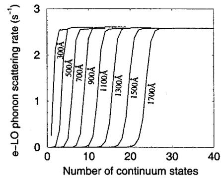
FIG. 3. An example of the total  $e-LO$  phonon absorption scattering rate from the bound state in a quantum well to the continuum as a function of the number of continuum states included in the summation at 77 K and for a variety of outer barrier widths.
