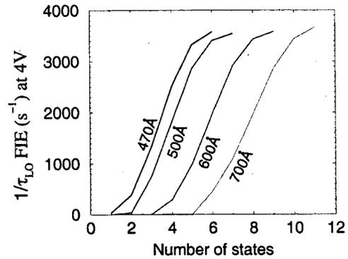
FIG. 10. Total  $e-LO$  phonon absorption scattering rate from the quantum well bound state to the continuum states as a function of the number of continuum states in the summation at 77 K, for four outer barrier widths at a bias of 4 V for the FIE component.
