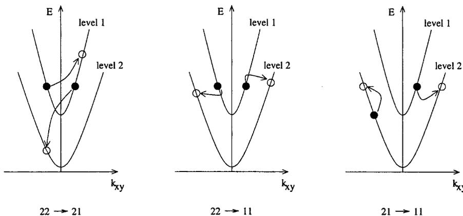
FIG. 2. Intersubband carrier–carrier scattering mechanisms in a two-level system (after Harrison Ref. 23): the solid circles represent the initial electron states, and the empty circles, the final states.
