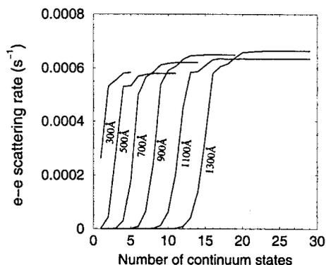
FIG. 4. An example of the total  $e-e$  scattering rate from the bound state in a quantum well to the continuum as a function of the number of continuum states included in the summation at 77 K and for a variety of outer barrier widths (as indicated on the figure).
