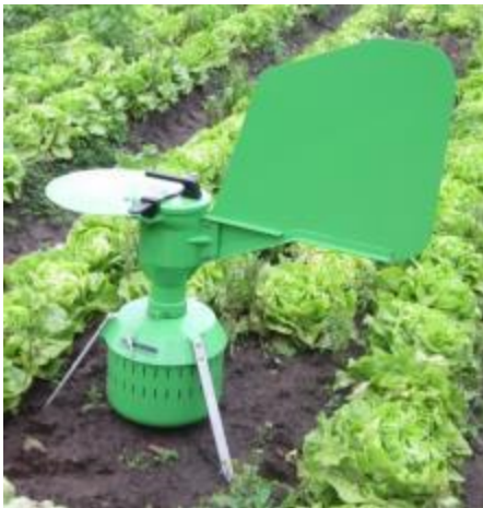
Figure 3-2: Volumetric spore sampling (Burkhard) set up in open field at PCG to monitor presence of B. lactucae conidia (picture from Aaike Bogaert).
