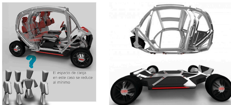
Fig. 18. Audi's compact spaceframe construction (aluminium tubular frame dressed with a carbon-fibre composite outer body, and mounted on a platform that integrates the battery pack).
