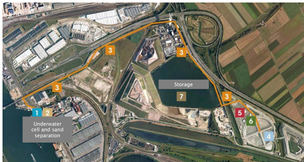
Fig. 1. AMORAS production sites: 1. underwater cell, 2. Sand separation, 3. Piping, 4. Consolidation ponds, 5. Dewatering installation, 6. Water treatment, 7. Storage.
