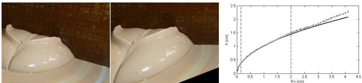
Fig. 8. Photo of the slump test used to measure the final profile, original (left) and after rectification (right). On the far right a digitalized profile (o) and its least square fit (solid line) is shown over the selected zone (between the vertical dashed lines).
