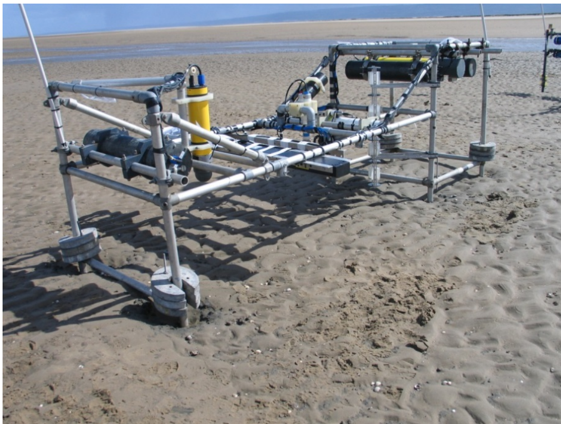
Fig. 5. SEDbed frame deployed at site 1, on the West Kirby tidal flats in the Dee Estuary.
