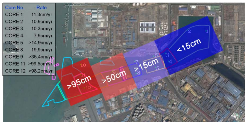
Fig. 2. Sedimentation rate in the North Harbour. The rate was evaluated with the core length divided by the year of sedimentation.
