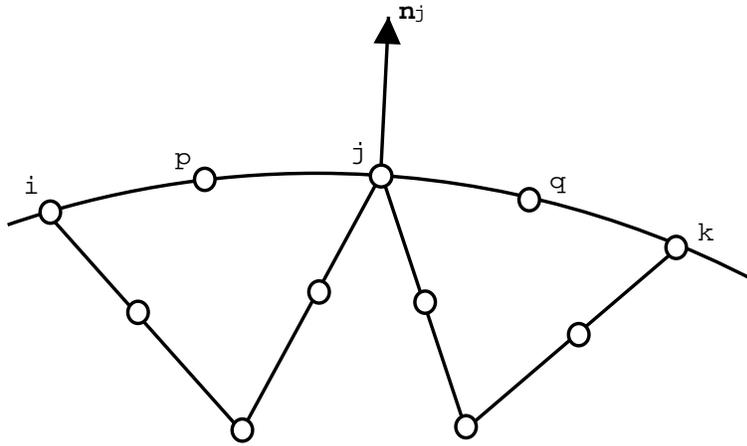
Figure 1. Isoparametric quadratic two-dimensional domain and boundary segment
