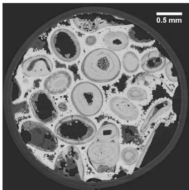
Fig. 5. Reconstruction using SPAR of a rock sample showing the remaining phase effects due to sample inhomogeneity.
