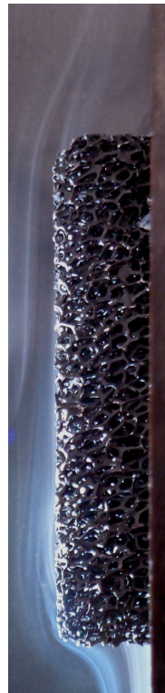
Figure 12. Visualization of the air flow through the in-house-made aluminum foam heat sink (reticulated22) using smoke ( \Delta T = 70 °C, vertical orientation).
