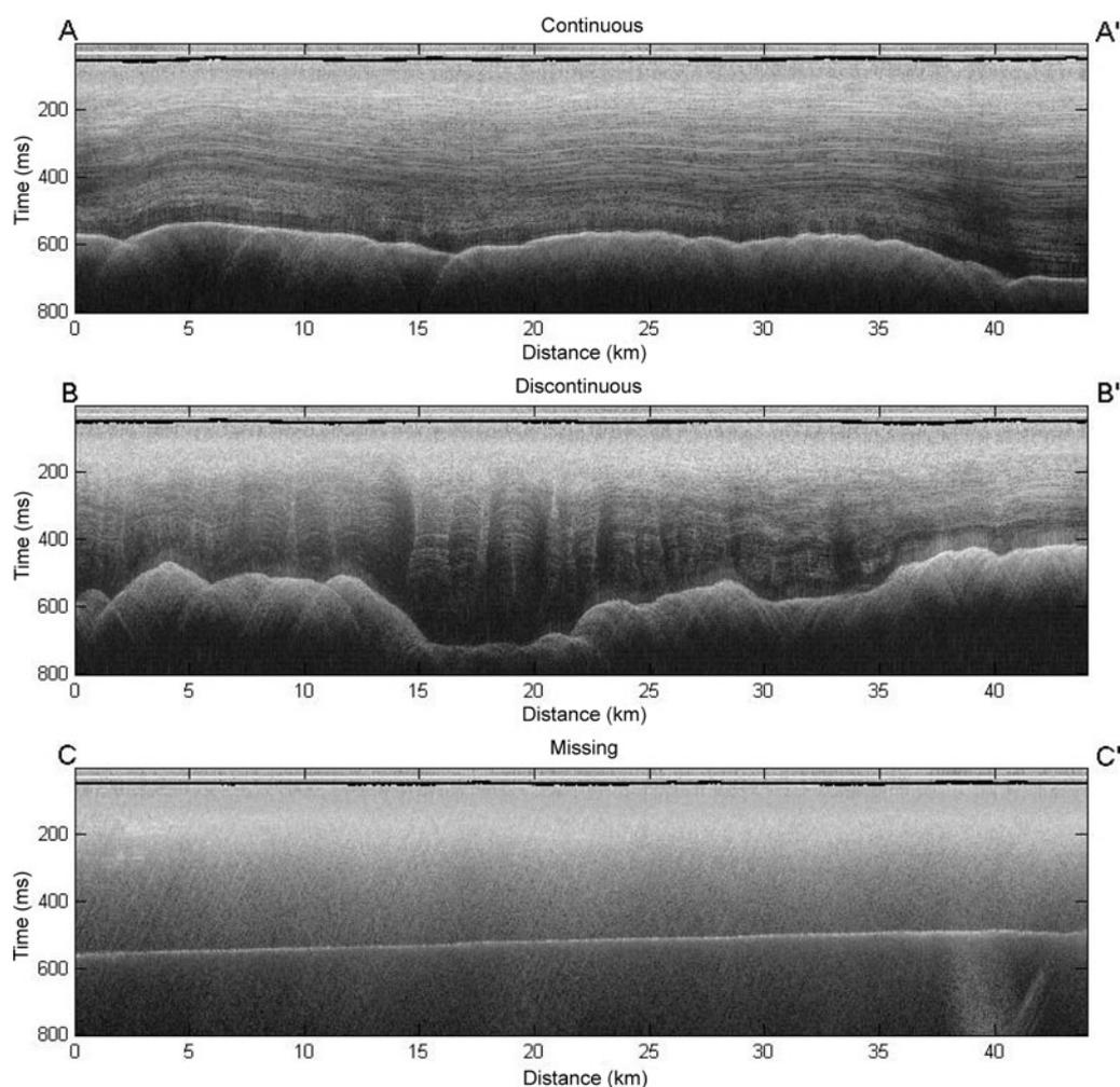
**Fig. 3.** Example of continuous (top), discontinuous (middle) and missing (bottom) layers. The thin black line marks the ice surface. The letters refer to the locations of the radargrams in Figure 4.
