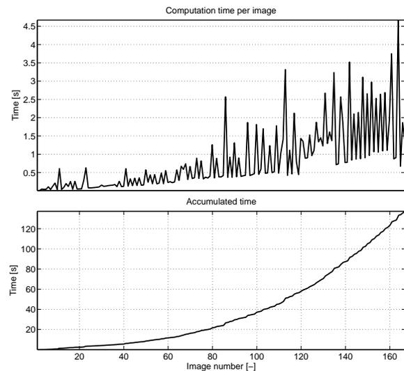
Fig. 9. Computation time per image and accumulated computation time for data set in Fig. 8, excluding feature computation and matching. The large deviation in computation time per image is due to that spectral clustering is not performed for every iteration, see Algorithm 2.
