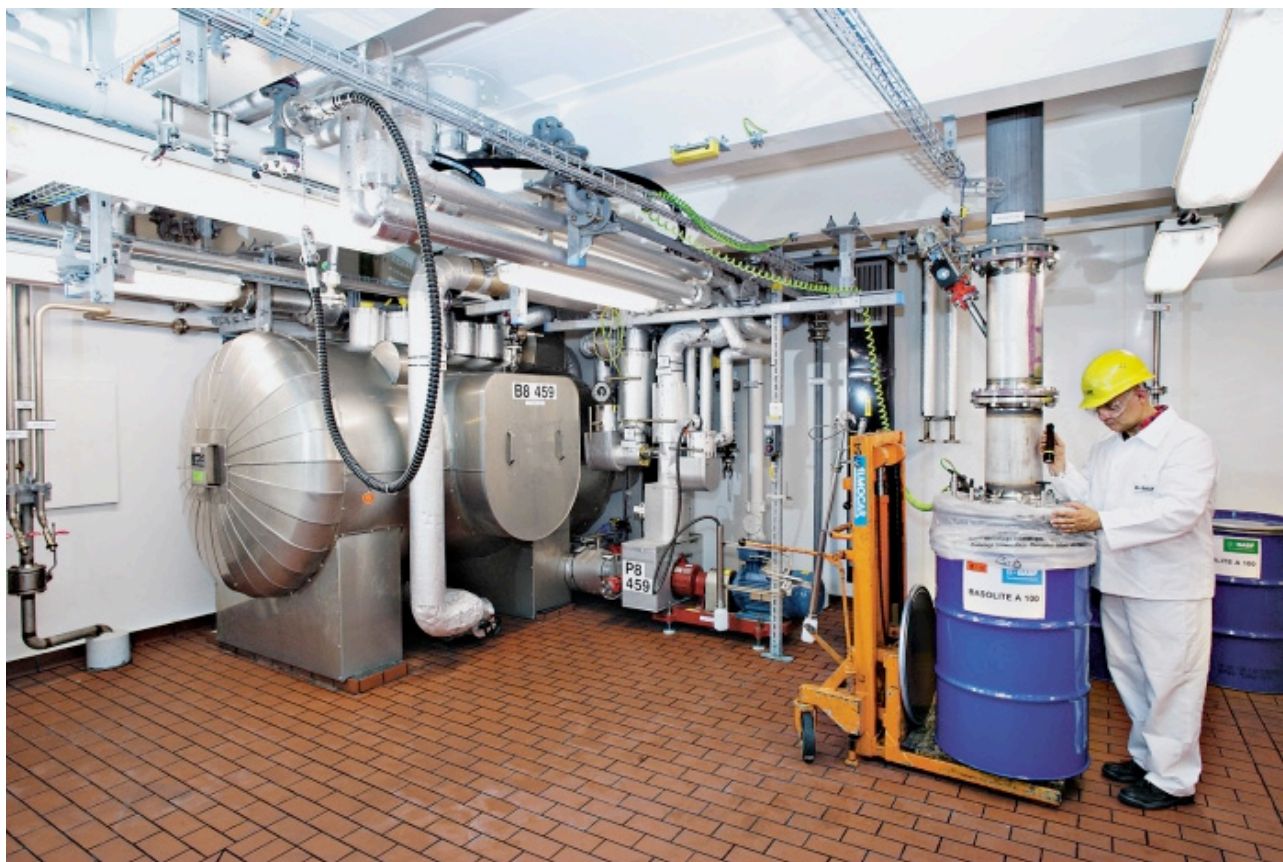
Figure 16 – Large-scale production of MOFs at BASF facilities in Germany. Image credit: BASF. (Reprinted with permission from ref. 210.)
