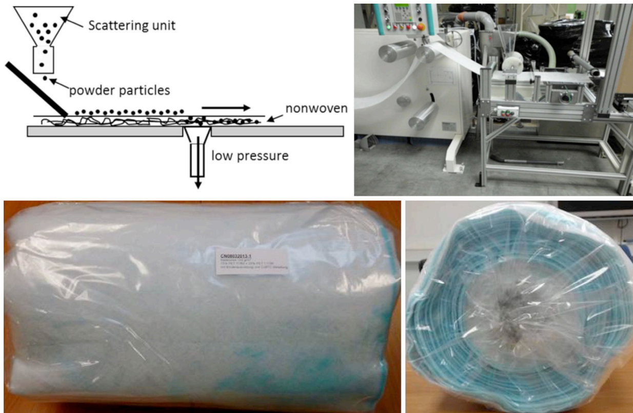
Figure 20 – Continuous and large-scale production process developed by Norafin in the context of NanoMOF project (reference FP7-NMP-2008-LARGE-2). ( Top left ) Principle of the dry loading process and ( top right ) the scattering-suction unit. ( Bottom ) Continuously MOF-particle loaded PET-nonwovens (HKUST-1 <math>63\ \mu\text{m}</math> from Johnson Matthey company; loading capacity: 25\ \text{g/m}^2 ). [Reprinted from http://cordis.europa.eu/project/rcn/92877_en.html (accessed 02 March 2015).]
