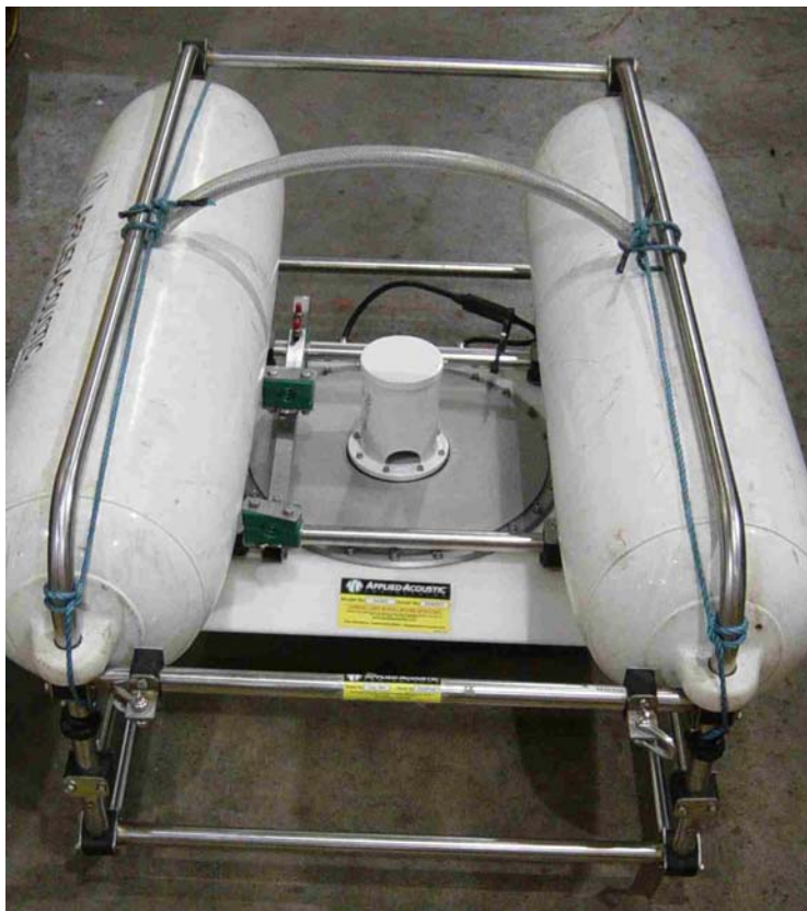
Applied Acoustics variable frequency S.T.Boomer Plate
