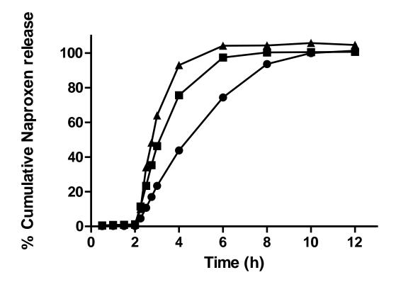
**Fig. 3.** *In-vitro* naproxen release profile of two extruded HPMC-AS-LF formulations with 30 (●) and 50 (■) % drug load. Dissolution in 0.1 N HCl (2 h) and pH 6.8 buffer (10 h) at 37 °C using paddle dissolution system at 100 rpm (Mean ± SD; n=3).
