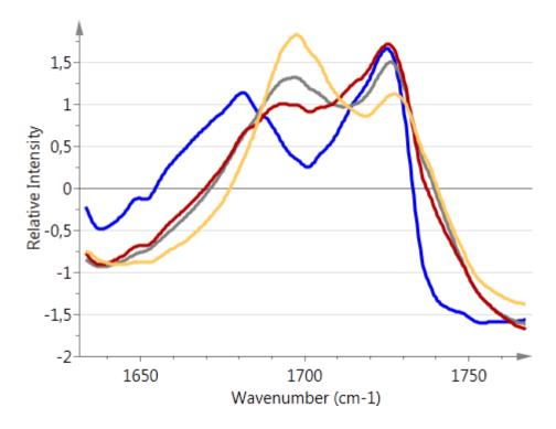
**Fig. 7.** ATR FT-IR spectra of naproxen (blue), HPMC-AS-LF (green), the physical mixture of HPMC-AS-LF plasticized with 10 % TEC and a drug load of 30% naproxen (red), the extrudate of the same formulation immediately after processing (yellow) and after storage for 2 weeks at 40 °C / 75 %RH (grey).
