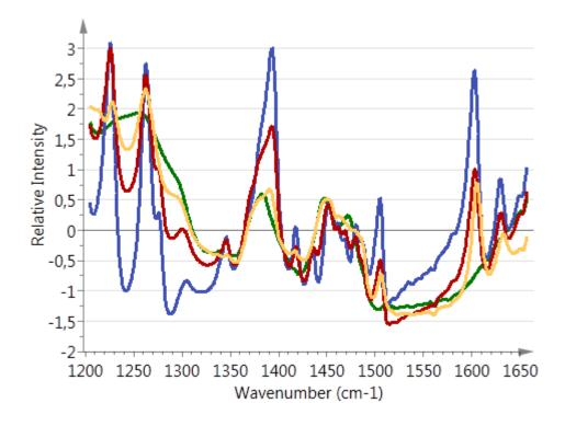
**Fig. 5.** ATR FT-IR spectra of naproxen (blue), physical mixture of Eudragit<sup>®</sup> L100-55 plasticized with 10 % TEC and a drug load of 30 % naproxen (red) and the extrudate of the same formulation immediately after processing (yellow) and after storage for 2 weeks at 40 °C / 75 %RH (grey).
