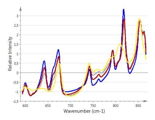
**Fig. 6.** ATR FT-IR spectra of naproxen (blue), physical mixture of Eudragit<sup>®</sup> L100-55 plasticized with 10 % TEC and a drug load of 30 % naproxen (red), the extrudate of the same formulation immediately after processing (yellow) and after storage for 2 weeks at 40 °C / 75 %RH (grey).
