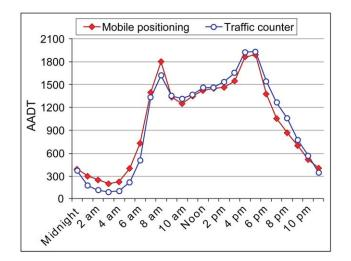
**Figure 3. The comparison of AADT between the traffic counter and mobile phone data.** The comparison of annual average daily traffic (AADT) between the stationary traffic counter data and estimated traffic flow extracted from the calibrated mobile phone data by hourly frequencies during the study period. doi:10.1371/journal.pone.0049171.g003
