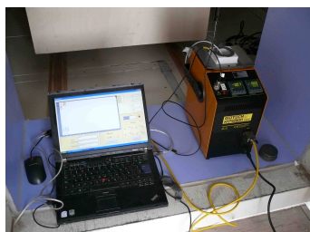
Calibrating temperature sensors in a controlled bath in the LCCE premises.
