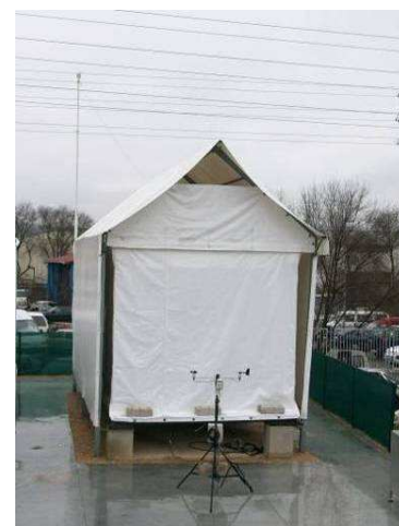
EGUZKI without sample and protected with a tarpaulin. Meteorological station is located 10 m high. Air temperature, velocity and direction in front of the sample.
