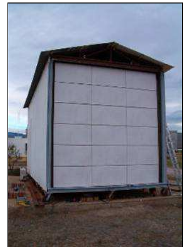
Ceramic ventilated façade being tested in a CESP test cell.
