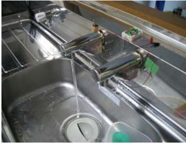
Automatically controlled tap: Amount of water is feedback controlled with flow meter by electromagnetic valves.
