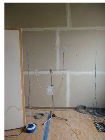
Radiation and temperature sensors on a measurement room in KUBIK
