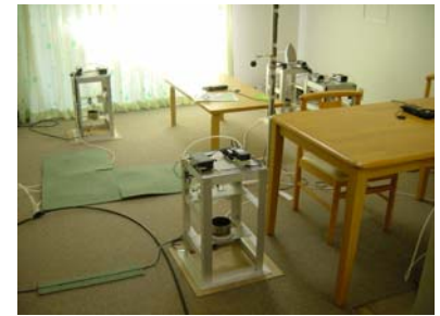
Heat and moisture generator for simulating occupants: Normally, total heat emission is set at 125W including latent heat of 38W (60g/h) in winter/medium seasons and 44W (70g/h) in summer season.
