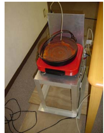
Heat and moisture generator for simulating cooking: Moisture of 74g/day and heat of 377kJ/day as a total for breakfast, lunch and dinner is normally set, according to the other experiments with subjects.
