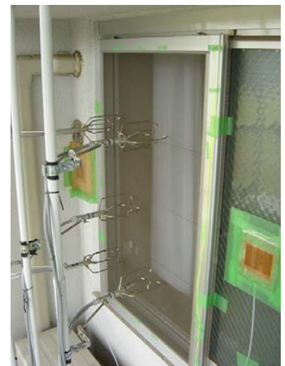
Example of the measurements. Exchanged air volume through the windows by cross ventilation is being measured by 3-dimensional ultrasonic anemometers besides windows. And the difference of the external pressure at each surface are also measured.
