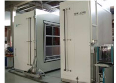
Test of building components in hot box.
