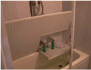
Controller for opening and closing bathtub cover plate: This simulates the degradation of the water temperature.
