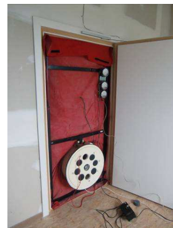
Air tightness test being performed in a measurement room in KUBIK
