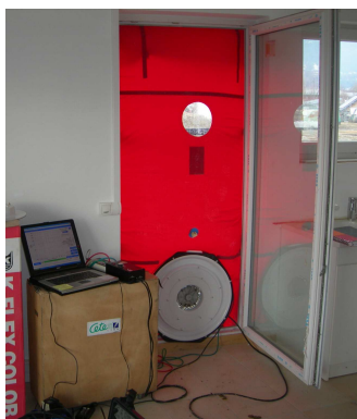
Airtightness test (blower door) in experimental houses.
