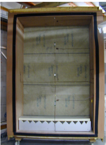
Semi Hot Box fitting a wall measurement bay in order to measure the overall U-value
