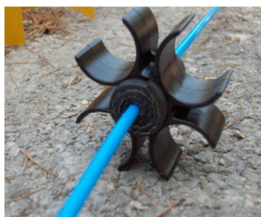
Location of the thermocouple using the pipes spacer
