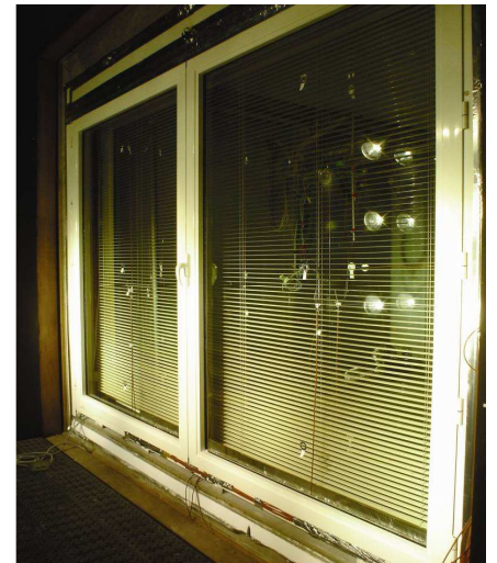
Double-Skin Façade tested on Minibat
