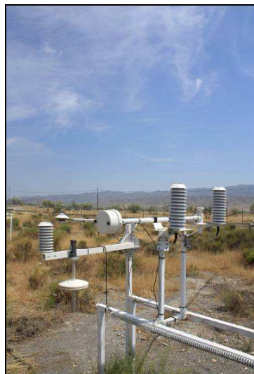
Different devices measuring outdoor air temperature, using natural and forced ventilation.
