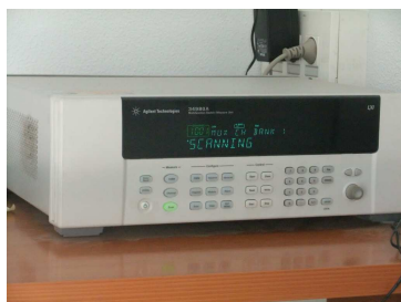
HP Agilent 34980A data acquisition system for logging and controlling the PASLINK tests.
