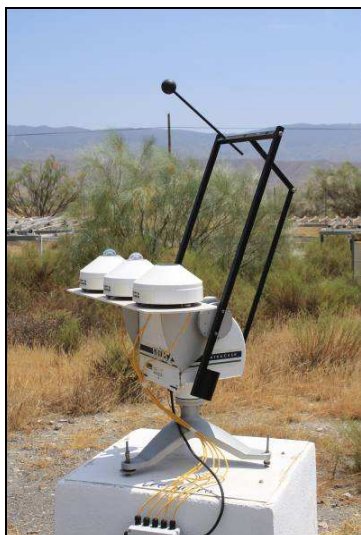
Device measuring solar global and diffuse, and longwave radiation.
