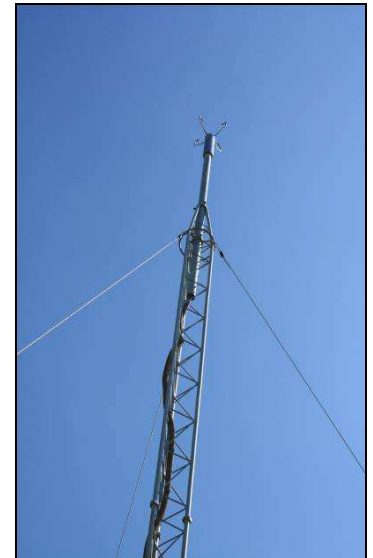
Ultrasonic device measuring wind speed and direction.
