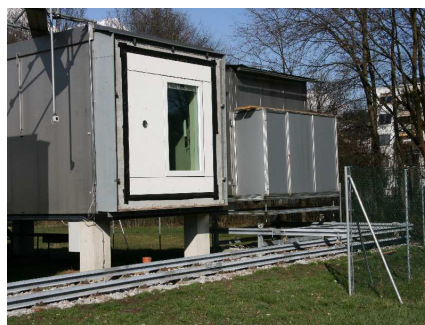
Testcell and Coldbox in parking position.
