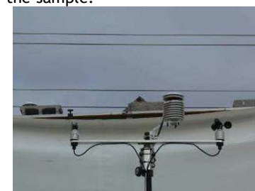
ILARGI air temperature, velocity and direction in the height of the roof.
