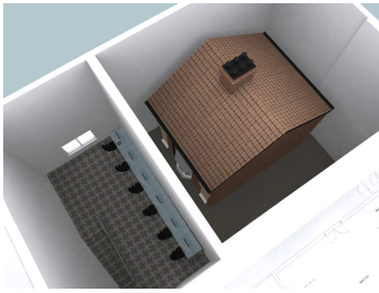
Salford Energy House in a fully environmentally controllable chamber.
