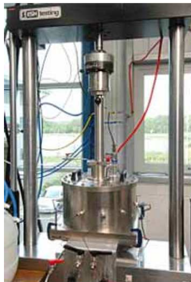
Figure 4: Corrosion fatigue crack growth rate equipment [10]
