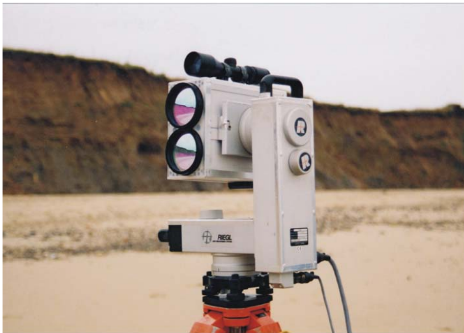
Figure 3 Riegl LPM-2K Long-range Terrestrial laser scanner.
