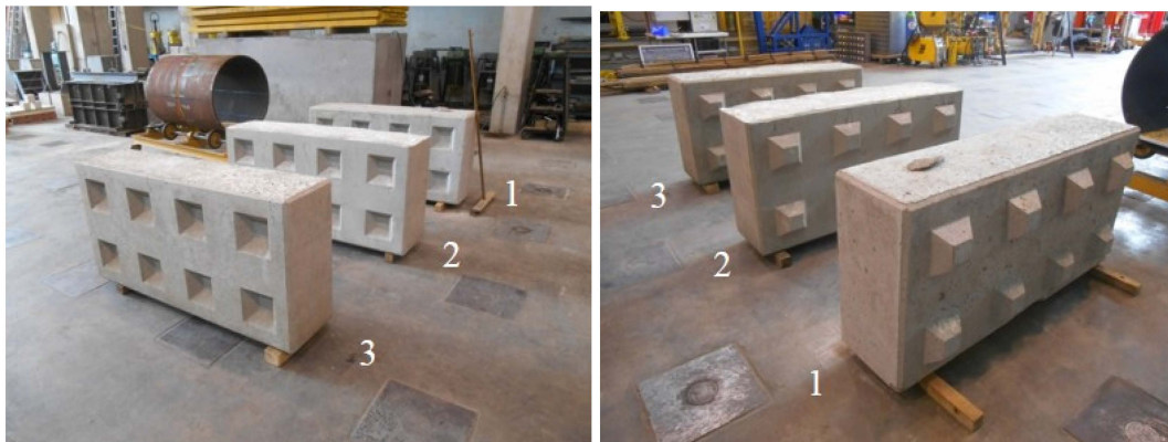
Figure 10. The three Lego bricks (3: the optimized BA-based Lego brick; 2: the reference limestone-based Lego brick; and 1: the BA-based unadjusted Lego brick).
