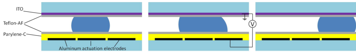
Figure 1. A diagram of the cross-section of an EWOD lab-on-a-chip and the electrowetting principle. When a voltage is applied to an actuation electrode, the droplet is attracted toward this activated region due to the generated imbalance in interfacial tension near the surface above the actuated electrode [16].
