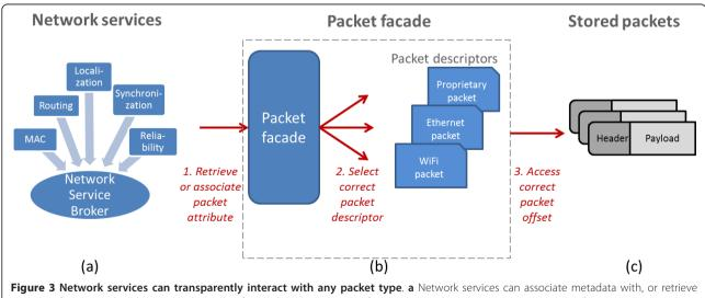
Figure 3 Network services can transparently interact with any packet type. a Network services can associate metadata with, or retrieve metadata from, stored packets using the packet facade. b Only the packet facade requires knowledge about the packet format. As long as the correct packet descriptor is available, the packet facade knows how and where metadata is stored. c Finally, the packet facade accesses the correct header offset or the packet payload.
