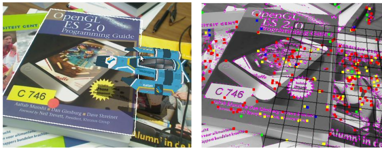
Figure 2: The augmented reality application tracks feature points in the video frames (right) to enable overlaying of 3D objects (left).
